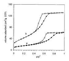
Fig. 3.  $N_2$  adsorption and desorption isotherms of (a) SN1 and (b) SN5 (filled mark, adsorption; empty mark, desorption) calcined at 723 K for 10 h.
