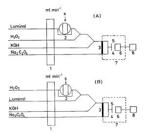
Fig. 1. Schematic diagram showing two configurations (A and B) of the flow-injection system used for the determination of pyridoxine hydrochloride and some of its pharmaceutical preparations; (1) peristaltic pump; (2) sample injection; (3) perspex T-piece; (4) waste; (5) coiled flow cell; (6) PMT; (7) housing; (8) recorder.
