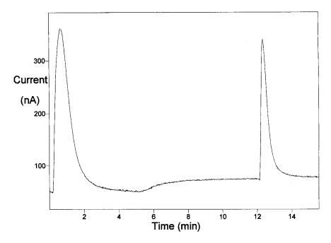
Fig. 3. Typical output data from the flow programming variation used to produce the data in Table 3. Flow injection analysis, both injections  $1 \times 10^{-3}$  M penicillin G. Solvent: 12% methanol/8% acetonitrile/80% 0.02 M acetate buffer (pH 4.7) (v/v). Flow program: initial flow, 0.5 ml min<sup>-1</sup>; final flow, 1.5 ml min<sup>-1</sup>; transition period, linear ramp between 5 and 6 min.
