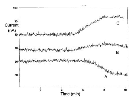
Fig. 5. Differing responses to an identical flow program for three different waveforms using the same solvent. Flow injection analysis. Flow program: initial flow, 1.0 ml min<sup>-1</sup>; final flow, 2.5 ml min<sup>-1</sup>; transition period, linear ramp between 5 and 8 min. Solvent: 0.02 M acetate buffer (pH 4.7). PAD waveform: given in Table 2A, except for E1 which was varied for each trace. Traces: (A) E1, 1350 mV, (B) E1, 1200 mV, (C) E1, 1050 mV.
