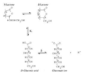
Fig. 1. Lactonitation and dissociation process of D-gluconic acid.  $\beta$  denotes the protolysis constant and  $K_r$  is the distribution constant.
