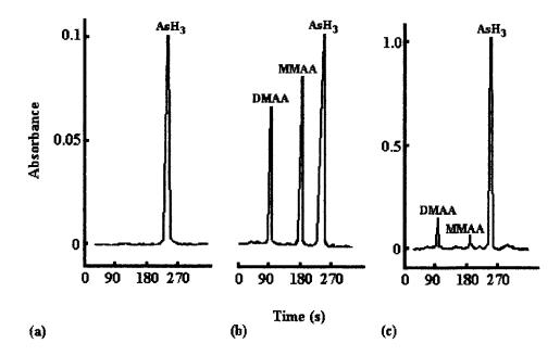
Fig. 3. Analytical signals obtained from inorganic arsenic (5 ng each) and its methylated species (10 ng each) using (a) 2 mol  $l^{-1}$  nitric acid and (b) 1% w/v citric acid. (c) This shows the responses from a trout fishery sample. The experimental conditions were as specified in Table 2.
