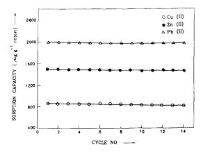
Fig. 5. Evaluation of the stability of Amberlite XAD-2-oVTSC for Cu(II), Zn(II) and Pb(II) loading and elution.
