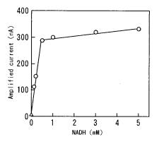
Fig. 3. Effect of NADH concentration in the carrier buffer on amplified current for  $1 \times 10^{-5}$  M L-glutamate.  $\Delta$ , without NADH.
