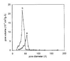
Fig. 4. BJH pore size distributions of (a) SN1 and (b) SN5 calcined at 723 K for 10 h.
