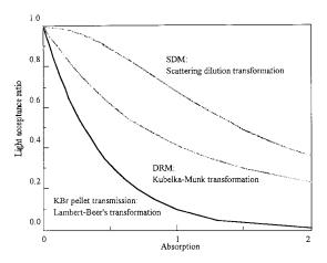
Fig. 19. Comparison of the transformation curve of SDM, DRM and transmission method.
