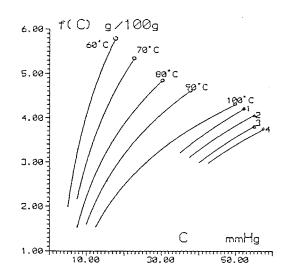
Fig. 2. Isotherms from 60 to 100°C silica gel (powder)—water, L = 50 cm,  $\Phi = 3/8$  inch,  $\omega = 2.5$  cc s<sup>-1</sup>, m = 0.500 ml. 1-Isotherms 100°C deduced from the chromatogram using formulas Eq. (4) and Eq. (5), 2-isotherm 100°C given by the manufacturer of the silica gel. 3-Isotherm 100°C deduced from [14], 4-isotherm 100°C deduced in [13].
