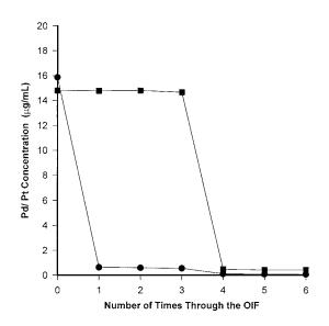
Fig. 11. Separation of Pt(IV) and Pd(II) using an OIF from a solution of 0.01 M  $NH_4SCN/0.73$  M HCl at a flow rate of 20 ml min<sup>-1</sup>. After the third pass through the filter the filtrate was exposed to UV light: •, Pd(II) concentration in filtrate; •, Pt(IV) concentration in filtrate.
