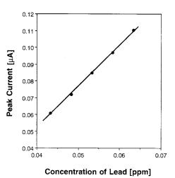
Fig. 5. Stripping signal vs. lead concentration in spiked whole blood samples measured with a bare mercury film electrode.
