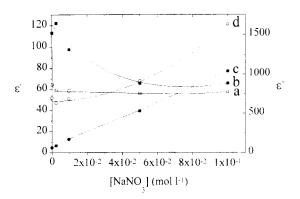
Fig. 4. Influence of the NaNO<sub>3</sub> concentration on the dielectric permittivity  $\epsilon'$  (curves **a** and **b**) and the dielectric losses  $\epsilon''$  (curves **c** and **d**) of 1.0 g silica gel in equilibrium with 10 ml of the NaNO<sub>3</sub> solution containing 0.46 M NH<sub>3</sub> (curves **b** and **d**) or not (curves **a** and **c**). Field frequency: 10 MHz.
