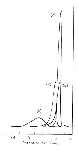
Fig. 3. Elution behaviors of (a)  $0.1 \ \mu g \ ml^{-1} V(V)$  solution, (b) 0.1  $\ \mu g \ ml^{-1} Fe(III)$  solution (c) 0.1  $\ \mu g \ ml^{-1} Fe(III)$  solution in the presence of 100  $\ \mu g \ ml^{-1} F^{-}$ , and (d) 0.1  $\ \mu g \ ml^{-1} Cu(II)$  solution.
