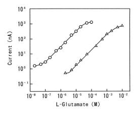
Fig. 5. Calibration graphs for L-glutamate: ( $\bigcirc$ ) Amplified current (obtained in the presence of NADH); ( $\triangle$ ) no amplified current (obtained in the absence of NADH). The carrier buffer [0.1 M ammonium phosphate buffer (pH 7.2) containing 3 mM NADH and 5 mM L-lysine] and Ringer's solution were pumped at 2 µl min<sup>-1</sup> in the flow system shown in Fig. 1(B).
