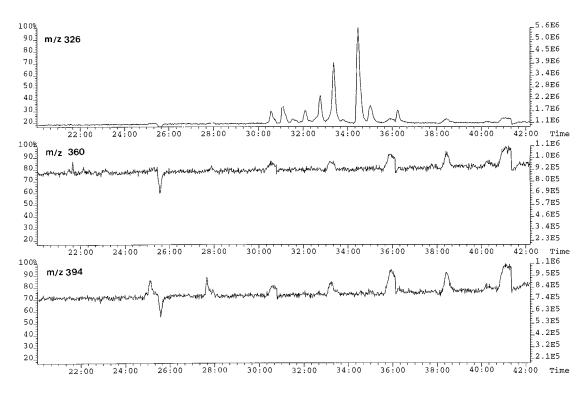
Fig. 1. NICI-GC-MS (single-ion monitoring) mass chromatograms (m/z = 326, 360 and 394, molecular ions for penta, hexa and hepta-chlorinated biphenyl, respectively) of the Loch Ness sediment sample after standard clean-up (see text). x-axis: retention time in minutes; y-axis: peak intensity.
