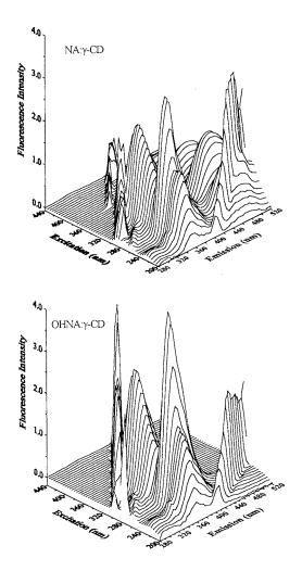
Fig. 1. Total luminescence spectra of the inclusion complexes of NA and OH–NA with  $\gamma$ -cyclodextrin. Each horizontal slice represents a separate emission scan with a fixed excitation wavelength.
