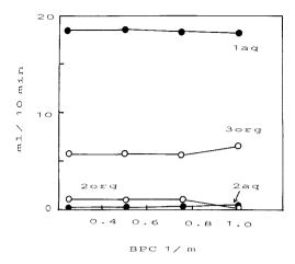
Fig. 3. Effect of BPC1 length sample: 200 µl; MG,  $1 \times 10^{-5}$  mol<sup>-1</sup>; buffer, pH 5; extraction coil, 0.5 m i.d. × 3 m; temperature, 20°C; flow rate, P<sub>1</sub> 1.94 ml min<sup>-1</sup>, P<sub>2</sub> 0.78 ml min<sup>-1</sup>;  $\lambda = 626$  nm; solvent, (toluene + MIBK = 1 + 1); BPC2, 6 m; BPC3, 0.5 m.
