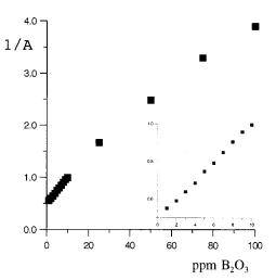
Fig. 2. Dependence between the inverse of the absorbance at 616 nm and the concentration of boric oxide in the conditions of Fig. 1. Bromocresol green was used as the indicator.
