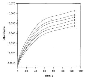
Fig. 4. Absorbance-time curves for the determination of the order of reaction with respect to vitamin C.  $[Fe^{3+}] = [H_2SO_4] = 2.162 \times 10^{-3}$  mol dm<sup>-3</sup>; [vitamin C] = (1)  $1.3810 \times 10^{-4}$ ; (2)  $1.5345 \times 10^{-4}$ ; (3)  $1.6879 \times 10^{-4}$ ; (4)  $1.8414 \times 10^{-4}$ ; (5)  $1.9948 \times 10^{-4}$ ; (6)  $2.1483 \times 10^{-4}$  mol dm<sup>-3</sup>; delay time,  $d_t = 12.0$  s.
