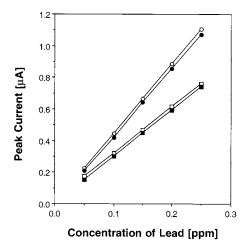
Fig. 7. Calibration plots for the modified electrodes with lead/EDTA and whole blood samples: ( $\bigcirc$ ) Nafion<sup>®</sup>-modified electrode; Pb<sup>2+</sup>/EDTA, ( $\bigcirc$ ) Cr<sup>3+</sup>/Nafion<sup>®</sup>-modified electrode; Pb<sup>2+</sup>/EDTA, ( $\square$ ) Nafion<sup>®</sup>-modified electrode; spiked whole blood, ( $\blacksquare$ ) Cr<sup>3+</sup>/Nafion<sup>®</sup>-modified electrode; spiked whole blood.
