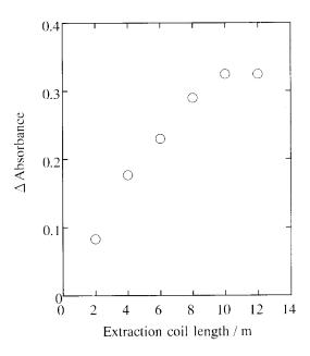
Fig. 7. Effect of extraction coil length on the FIA peak heights for silver(I). [Ag<sup>I</sup>],  $5.0 \times 10^{-7}$  mol dm<sup>-3</sup>. Conditions as in Fig. 1.
