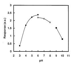
Fig. 4. Dependence of biosensor response on pH in 1 mM glucose solution at 25°C. ( $\bullet$ ) 0.1 M citrate, ( $\bigcirc$ ) 0.1 M phosphate and ( $\blacksquare$ ) 0.1 M carbonate buffer.
