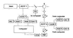
Fig. 1. Schematic diagram of the AOTF based fluorimeter: PD, photodiode; S, sample; P, polarizer; PMT, photomultiplier tube; amp, amplifier; osc, oscillator; mod, modulator; comb, combiner.
