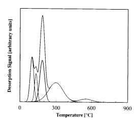
Fig. 7. Deconvolution of the TPDE signal for  $[Mo(CO)_6]$  on alumina pretreated to 1000°C.
