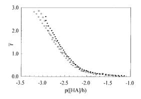
Fig. 5. Formation curves obtained for the Ni(II)/PAA  $3 \times 10^{6}$  system with different values of *R*: •, 3.2;  $\bigcirc$ , 6.4;  $\square$ , 12.7 (*C*<sub>A</sub> = 5.1 meq 1<sup>-1</sup>).
