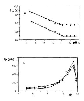
Fig. 2. Influence of pH on: (a) half-wave potential in DC-polarography and (b) peak current in DPV, for a  $1 \times 10^{-7}$  mol  $1^{-1}$  Nitralin solution with its optimum working conditions. First wave ( $\bullet$ ) and second wave ( $\Box$ ).
