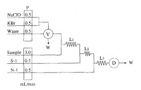
Fig. 1. Schematic diagram of the FIA dystem for determination of ammonia. P, peristaltic pump; V, injection valve; D, detector;  $L_1$ ,  $L_2$ ,  $L_3$ , reaction tube; S-1, sulfanilamide solution; N-1, N-1-naphthylethylenediamine solution; W, waste.
