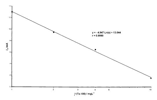
Fig. 1. Calibration curve for Triton X-100 in a supporting electrolyte containing NaCl and HgCl<sub>2</sub>.
