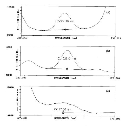
Fig. 5. ICP optical emission spectrum registered aspirating 1 mg  $1^{-1}$  of Co (a), Cu (b) and P (c).
