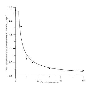
Fig. 3. The change of concentration of surface active substances in river water (in equivalents of Triton X-100) with ozonolysis time.
