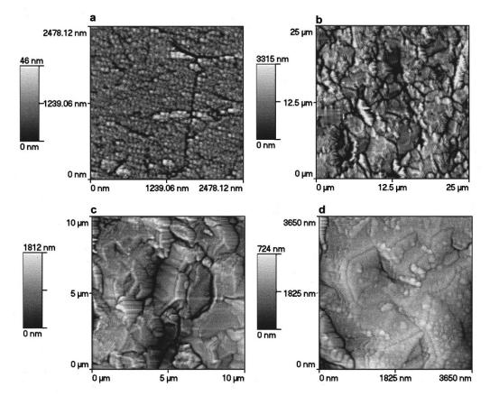
Fig. 4. AFM images of the uncoated QCM and coated QCM. (a)  $2500 \times 2500$  nm region; (b)  $25 \times 25 \mu$ m AFM images of 20-layer LB films on QCM; (c) 10  $\mu$ m ×  $\mu$ m, enlarged area of the middle of (b); (d)  $3650 \times 3650$  nm, enlarged area of the upper left of the (c).
