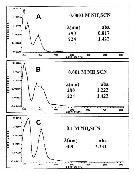
Fig. 4. The UV/Vis spectra of solutions containing 5  $\mu$ g ml<sup>-1</sup> Pd and 0.73 M HCl and various concentrations of NH<sub>4</sub>SCN. A,  $1 \times 10^{-4}$  M NH<sub>4</sub>SCN; B,  $1 \times 10^{-3}$  NH<sub>4</sub>SCN; C, 0.1 M NH<sub>4</sub>SCN.
