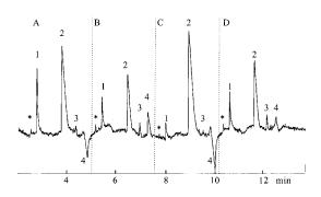
Fig. 7. Determination of carbonate and free SO<sub>2</sub> in wine samples. Valve actuations at t = 0, 2.5, 5 and 7.5 min. Peaks: 1, SO<sub>3</sub><sup>2-</sup>; 2, HCO<sub>3</sub><sup>-</sup>; 3, acetate; \*, SO<sub>4</sub><sup>2-</sup>. Samples: A, white wine 1; B, white wine 2; C, red wine 1; D, red wine 2. Conditions as in Fig. 3.
