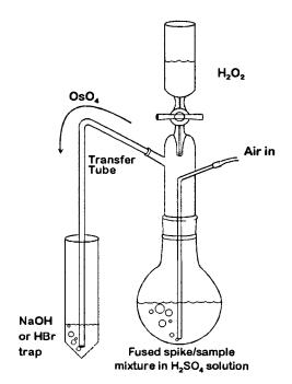
Fig. 1. Apparatus for distillation of Os.
