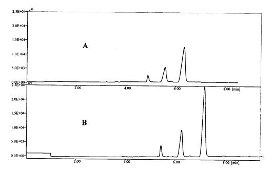
Fig. 3. Effect of electrolytes on the separation of benzyl penicillin (Pen G), 6-APA, and phenyl acetic acid. (A) 20 mM Na<sub>2</sub>PO<sub>4</sub> (pH 9.0); (B) 20 mM borate (pH 8.9). Injection, 10 s/10 cm by gravity; capillary column, fused silica/55 cm total length/43 cm effective length/50  $\mu$ m I.D.; voltage, 15 kV; UV detection, 210 nm.
