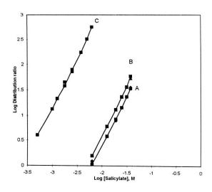
Fig. 3. Plots of log of distribution ratio vs. log of salicylate concentration for trivalent gallium (A) (at fixed pH 6.5 and 10 ml of 0.15% TPASO), indium (B) (at fixed pH 5.0 and 5 ml of 0.5% TPASO) and thallium (C) (at fixed pH 3.0 and 5 ml of 0.3% TPASO).
