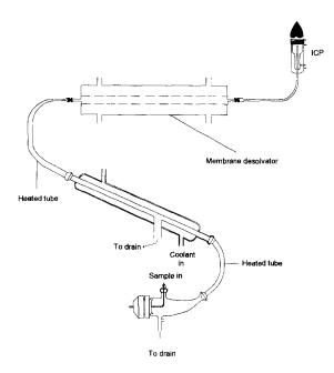
Fig. 2. General system diagram.
