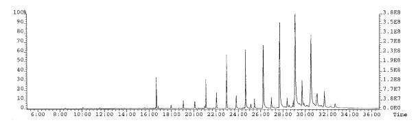
Fig. 2. Total ion chromatogram of the Loch Ness sediment sample analysed in full scan electron impact mode, showing a typical higher plant n-alkane distribution. x-axis: retention time in minutes; y-axis: peak intensity.
