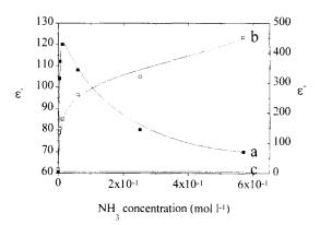
Fig. 5. Influence of the ammonia concentration on the equilibrium values of dielectric permittivity  $\epsilon'$  (a) and the dielectric losses  $\epsilon''$  (b) of silica gel. The dielectric permittivity  $\epsilon'$  of silica gel in pure water (c) was added for comparison purpose. Field frequency: 10 MHz.
