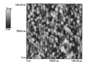
Fig. 4. AFM image of SM3 latex particles. The AFM images were obtained in non-contact mode.
