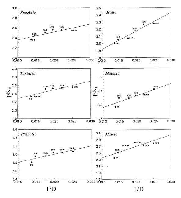
Fig. 4.  $pK_D-1/D$  correlation for the ion-pair association reaction of dicarboxylic acids in different solvent compositions at 40°C.
