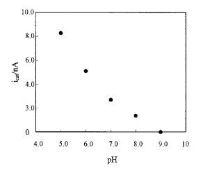
Fig. 5. The dependence of catalytic currents on pH from CVs in  $2.0 \times 10^{-3}$  M ascorbic acid phosphate buffer solution at scan rate of 10 mV s<sup>-1</sup>.
