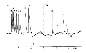
Fig. 3. Separation of a model anion solution (A) without and (B) with gas diffusion. Conditions: electrolyte I (chromate); 25 kV; acceptor solution: 5 mmol  $1^{-1}$  tris. The injection valve was actuated at t = 0 (A) and at t = 3 min (B). Peaks: 1,  $S_2O_3^{2-}$ ; 2,  $CI^-$ ; 3,  $SO_4^{2-}$ ; 4,  $NO_3^-$ ; 5,  $HS^-$ ; 6,  $SO_3^{2-}$ ; 7, citrate; 8, fumarate; 9, formate; 10,  $HCO_3^-$ ; 11, acetate. Flow rates according to Fig. 2.
