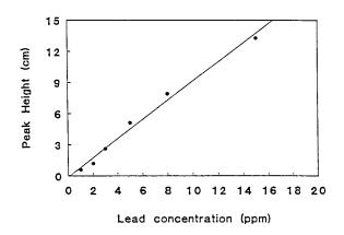
Fig. 7. Stripping peak heights of Pb(II) measured by a peat moss electrode for different Pb(II) concentrations.
