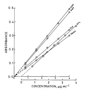
Fig. 3. Beer's law plots of amoxycillin (AMX), ampicillin (AMP), cloxacillin (CLX), cefadroxil (CFL) and penicillin V (PEN V) with I<sub>2</sub>–WFB system. [I<sub>2</sub>],  $9.45 \times 10^{-5}$  M; [WFB],  $7.82 \times 10^{-5}$  M; [NaOH],  $8.0 \times 10^{-2}$  M.
