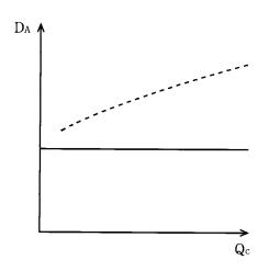
Fig. 13. Relationship between axial dispersion  $D_A$  and flowrate  $Q_c$ . Solid line: Without the dispersion, Dotted line: With the dispersion.
