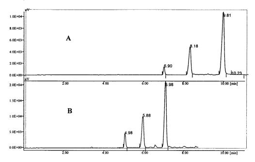
Fig. 6. Effect of capillary length on the migration time. (A) Capillary with 55 cm total length/43 cm effective length; (B) capillary with 50 cm total length/38 cm effective length. Other conditions of electrophoresis were the same as described in Fig. 3.
