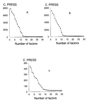
Fig. 2. Representation of the cumulative PRESS vs. the number of principal components for the PLS-1 modelling. a) With no preprocessing of the raw data, b) the raw data were scaled against the mean, and, c) the raw data were scaled against the mean and the standard deviation.
