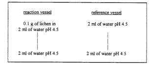
After 30 min of thermal equilibration, the calorimetric unit was rotated and the heat output was recorded and monitored for at least 30 min. During the trace recording, the calorimeter drum was rotated at a 10-min interval to minimize lichen sedimentation inside the calorimetric vessel. The lichen-derived heat production was calculated by considering that the instrument output is directly related to the heat evolved inside the calorimeter:
