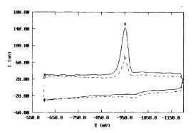
Fig. 1. Cyclic voltammograms of NiTMpyP (a)  $1 \times 10^{-6}$  M and (b) mixture of  $1 \times 10^{-6}$  M NiTMpyP with  $2 \times 10^{-6}$  M DNA. Background electrolytes 0.1 M HAc–NaAc, pH 5.8; accumulation time  $t_A = 2$  s; accumulation potential  $E_A = -0.6$  V; switching potential  $E_{SW} = -1.2$  V; scan rate 0.2 V s<sup>-1</sup>.
