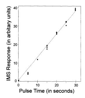
Fig. 6. Plots of IMS response to TNT pulsed from the vapor generator at 79°C. Response was obtained by integrating plots of the peak intensities for the product ion of TNT in the negative mode (see Fig. 8) versus time.
