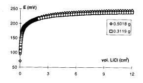
Fig. 1. Potentiometric titrations obtained for the  $H^+$ -Li<sup>+</sup> system in Dowex CM-15. The legend indicates the grams of the resin in the proton form.
