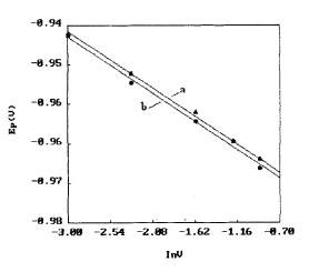
Fig. 5. Semilogarithmic dependence of the peak potential  $E_p$  on the potential scan rate ln  $\nu$ : for (a)  $1 \times 10^{-6}$  M NiTMpyP pH 5.8; (b) a + 1 × 10<sup>-6</sup> M DNA.
