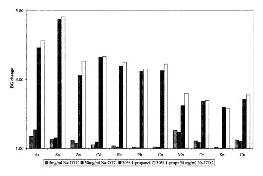
Fig. 3. Matrix induced change of the background emission on Na-DTC and 1-propanol normalised to RDW.
