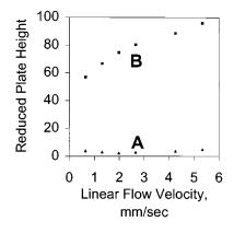
Fig. 3. Reduced plate height, h, as a function of linear flow velocity, u, on a brush-type WRP column for the unretained analyte benzoic acid (A) and a retained analyte ethyl benzene, k = 1 (B). A linear flow velocity of 2.7 mm s<sup>-1</sup> corresponds to a volumetric flow rate of 1.0 ml min<sup>-1</sup>. The column dimensions and detection were the same as in Fig. 2.
