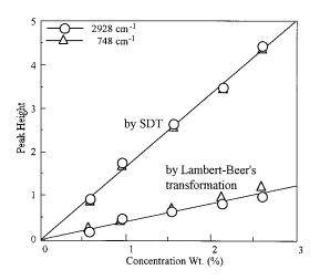
Fig. 20. Comparison of carribration curves by SDT and by Lambert–Beer's transformation.
