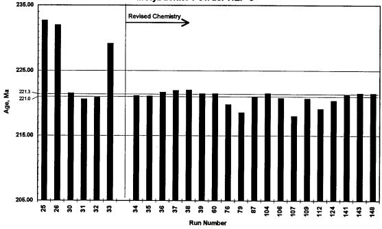
Fig. 2. Histogram illustrating the improvement in reproducibility of our method after revising the chemical procedure described in Ref. [9]. All analyses are for HLP-5.
