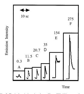
Fig. 2. Typical emission signals at silicon 251.611 nm produced by standard silicon solution: A, blank; B, 1; C, 5; D, 10; E, 50; F, 100  $\mu$ g ml<sup>-1</sup> silicon. The numbers next to the peaks are peak-height measurements in cm.
