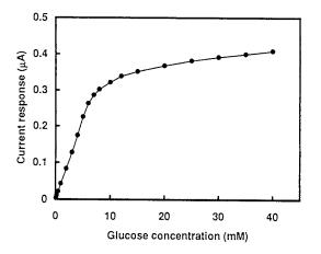
Fig. 3. Calibration graph for glucose obtained at pH 6.0 and 25°C.
