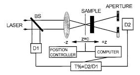
Fig. 1. Schematic diagram of the experimental setup for Zscan measurements in which the energy ratio is recorded as a function of the sample position z. The abbreviations are: BS, beam splitter; D1 and D2, energy detectors.
