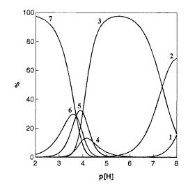
Fig. 3. Distribution curves for the 1:2 TC18C6-2Al<sup>3+</sup> system. 1, Al<sub>2</sub>L(OH)<sub>4</sub>; 2, Al<sub>2</sub>L(OH)<sub>3</sub>; 3, Al<sub>2</sub>L(OH)<sub>2</sub>; 4, Al<sub>2</sub>L(OH); 5, Al<sub>2</sub>L; 6, Al<sub>2</sub>HL; 7, Al<sub>2</sub>H<sub>2</sub>L.
