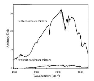
Fig. 16. Improvement in detection efficiency of lights transmitted and scattered.
