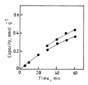
Fig. 5. Interruption test. 0.1 g resin, pH 5, 25 cm<sup>3</sup> reaction volume, equilibration time 24 h, copper, concentration 200  $\mu g$  cm  $^{-3}.$
