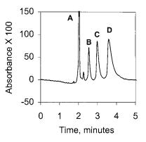
Fig. 2. WRP-LC separation of 10  $\mu$ l sample containing 10 ppm benzaldehyde (A), 5 ppm benzene (B), 5 ppm toluene (C), 10 ppm ethyl benzene (D) with a water mobile phase at a flow rate of 0.75 ml/min on a 4.6 mm  $\times$  250 mm branched WRP column. Detection was done with UV absorbance at 200 nm.
