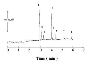
Fig. 10. The electropherogram of the eight standard anion mixture near the limit of detection using the hydrodynamic sampling. Conditions: BGE: 5 mM Molybdate, 0.15 mM CTAH, 0.01% PVA and 5 mM Tris buffer at pH 7.9; Capillary: 65 cm  $\times$  0.075 mm i.d. fused silica; Run: -20 kV; Injection: 8 cm for 60 s; Detection: 230 nm; Current: 10  $\mu$ A. Anion standards: 200 ppb each: 1 = chloride; 2 = sulphate; 3 = nitrate; 4 = fluoride; 5 = formate; 6 = phosphate; 7 = carbonate; 8 = acetate.
