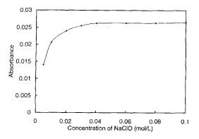
Fig. 2. Influence of concentration of sodium hypochlorite. Other reagents concentration: 15% potassium bromide in 4 M sodium hyroxide; injection volume:  $350 \mu$ l.
