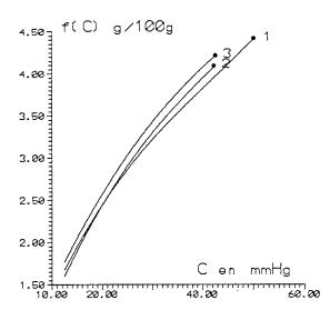
Fig. 13. Isotherms 100°C silica gel (powder)-water, L = 50 cm,  $\Phi = 3/8$  inch, m = 0.500 ml,  $\omega = 2.5$  cc s<sup>-1</sup> (1), 5 cc s<sup>-1</sup> (2), 1 cc s<sup>-1</sup> (3).
