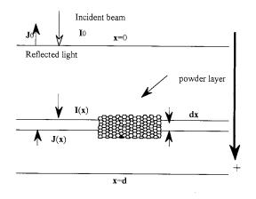
Fig. 18. Kubelka-Munk's model of different powder's layer.
