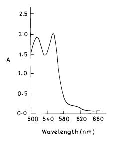
Fig. 1. Zero-order spectrum of Ir-PAN-naphthalene in DMF. Ir: 25 µg; PAN: 1.0 ml (0.1%); pH: 5.5; naphthalene: 2.0 ml (20% in acetone); reference: reagent blank.
