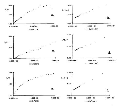
Fig. 4. Typical Stern-Volmer plots for the experiments with csFA and (a, b) Cu(II), (c, d) Fe(III) and (e, f)  $UO_2^{2+}$ : (a, c, e) original Stern-Volmer plots; and (b, d, f) modified Stern-Volmer plots.
