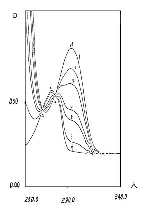
Fig. 1. Absorption spectra of L-tyrosine at  $298.2 \pm 0.2$  K at constant total ionic strength, 0.1 mol kg<sup>-1</sup>, and various pH values (from top to bottom): (1) 11.832, (2) 10.356, (3) 0.863, (4) 9.602, (6) 9.362, (6) 8.647, (7) 4.806. *D* means absorbance.
