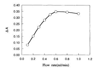
Fig. 4. Effect of flow rate. Concentration of  $SO_4^{2-1}$ : 4 mg  $l^{-1}$ ; injection volume: 200 µl.
