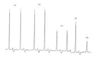
Fig. 5. Typical signal traces for (a) river water, (b) seawater, (c) 1.0 ng ml<sup>-1</sup> vanadium standard solution, (d) 2.0 ng ml<sup>-1</sup> vanadium standard solution and (e) seawater spiked with 0.50 ng ml<sup>-1</sup> vanadium by the present FIA system using a 5 m sample loop injection.
