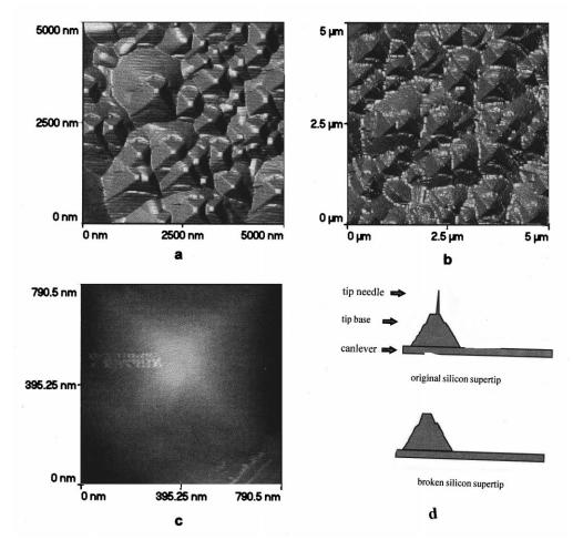
Fig. 3. Images for the broken supertip showing the tip base in truncated pyramidal shape. Note the flat terrace on top of the feature and the covered structure of the lower half of the feature. (a) Tip image obtained in contact mode; (b) tip image obtained in noncontact mode; (c) tip image obtained by scanning the tip over single vertical crystallite in noncontact mode. Note the bright round spot, corresponding to the broken scar of the tip needle; (d) a diagram of the supertip.
