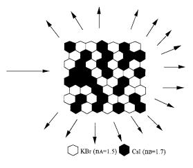
Fig. 8. Idea of mixed powders' pellet having different n components (nA, nB) for scattering media.
