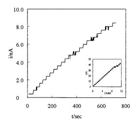
Fig. 6. Dynamic response of the composite polymer modified electrode to successive addition of ascorbic acid in 0.1 mM steps at a constant potential of 0.2 V vs. SCE in pH 7.0 buffer solution. Insertion: the corresponding calibration curve.
