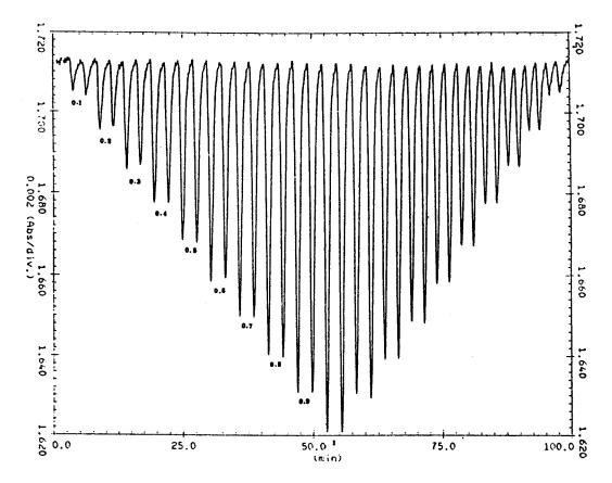
Fig. 6. FIA signals obtained at varing nitrite concentration. The numbers on the peaks show the concentration of nitrite in  $\mu$ g ml<sup>-1</sup>.
