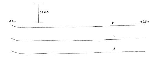
Fig. 8. Stripping-mode voltammograms of Pb(II) in a water sample from Contraband Bayou measured by a peat moss electrode.
