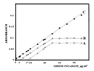
Fig. 2. Calibration curves for cyclamate obtained with different concentrations of ethanol as washing solution: A, 10%; B, 20%; C, 30%. Dissolving solution: 0.5 M ammonium acetate.
