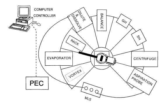
Fig. 1. Robotic station for TCP leaching from soil and fruit. MLS denotes master laboratory station; GH, general hand; SH, syringe hand; PEC, power and even controller.
