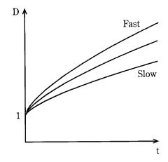
Fig. 8. Relationship between radial dispersion D and residence time t at various flow-rate.
