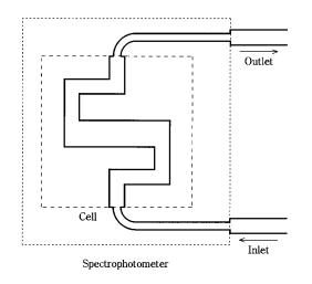
Fig. 3. Construction of flow-through cell for spectrophotometer.
