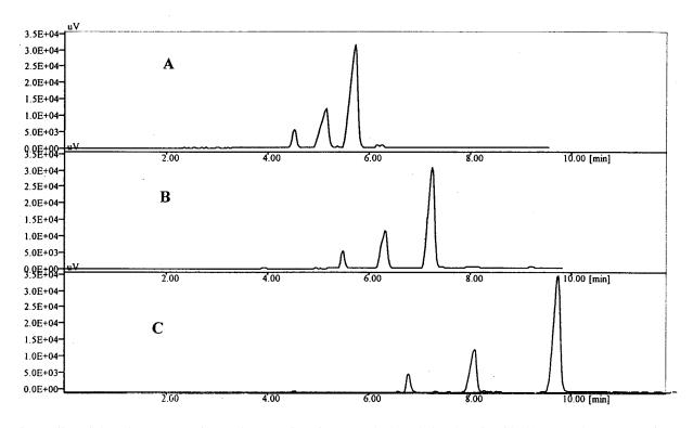
Fig. 5. Effect of electrolyte concentration on the separation of Pen G, 6-APA, and phenyl acetic acid. (A) 10 mM borate as running buffer; (B) 20 mM borate as running buffer; (C) 40 mM borate as running buffer. Other conditions of electrophoresis were the same as described in Fig. 3.
