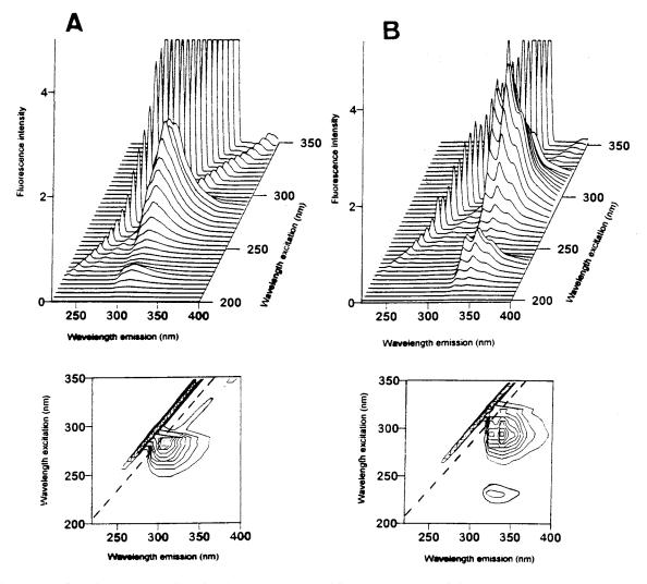
Fig. 1. Three-dimensional and two-dimensional (contour plots) total fluorescence spectra of pindolol (A) and propranolol (B). Other conditions as in figure  $C_{PIN} = 10 \text{ } \mu\text{mol } 1^{-1}$ .
