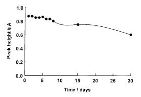
Fig. 4. Biosensor stability. The biosensor was based on RVC coated with immobilised acetylcholine esterase. At the times indicated the biosensor response to substrate was checked as in Fig. 3.
