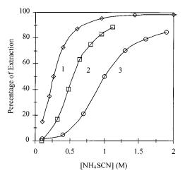
Fig. 2. Percentage of extraction of Co(II) at equilibrium, at  $25 \pm 2^{\circ}$ C, as a function of NH<sub>4</sub>SCN concentration by MIBK (98%), in absence (1) and presence of H<sub>2</sub>SO<sub>4</sub> 1 M (2) and 2 M (3). Phase ratio = 1. [Co(II)] was initially  $10^{-3}$  M.
