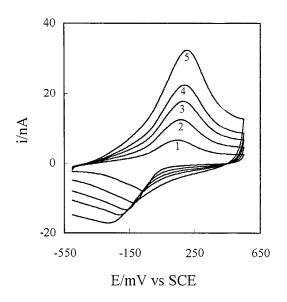
Fig. 3. The cyclic voltammograms at the composite polymer modified electrode in pH 7.0 buffer solution at the scan rate: (1) 10; (2) 30; (3) 50; (4) 70 and (5) 9O mV s<sup>-1</sup>.
