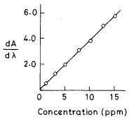
Fig. 4. Calibration curve for Ir by first order spectrophotometry from signal peak to peak measurements between  $\lambda_1 = 565$  and  $\lambda_2 = 543$  nm ( $\Delta \lambda = 10$  nm). Rest of the conditions same as Fig. 2.
