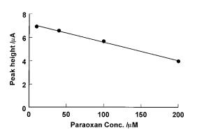
Fig. 6. Pesticide determination with RVC-agarose composite electrode. The analysis was carried out in a continuous, competitive FIA mode. The transporting buffer contained besides the electron mediator the substrate acetylthiocholine (0.4 mM). Samples of paraoxon (0.1 ml) at the concentrations indicated were injected and the decreased response level was recorded.
