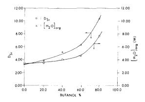
Fig. 1. Distribution ratio of  $Sr^{2+}$  and the organic phase water content as a function of increasing butanol content in butanol-octanol mixture; [DCH18C6] = 0.1 M; [HNO<sub>3</sub>]<sub>aq</sub> = 4.05 M.
