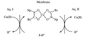
Fig. 4. Schematic representation of the reactions taking place at the boundary of the source phase and the chloroform and at the boundary of the chloroform and the receiving phase.
