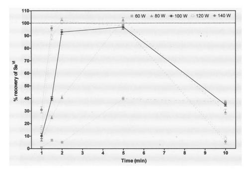
Fig. 2. Se<sup>VI</sup> recovery obtained in a focused microwave device (Working concentration 1  $\mu$ g l<sup>-1</sup> as Se content; HCl concentration 6 mol l<sup>-1</sup>).
