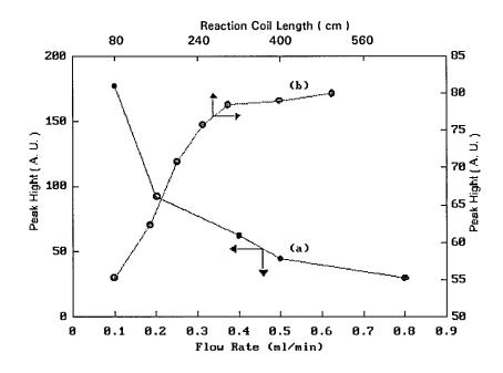
Fig. 4. Effects of flow rate (a), and reaction coil length (b), on the peak height. Conditions: safranine 12  $\mu$ g ml<sup>-1</sup>; KCl, 0.06 M; nitrite, 0.8  $\mu$ g ml<sup>-1</sup>; HCl 0.16 M;  $T = 25^{\circ}$ C; sample loop volume, 110  $\mu$ l; and flow-rate, 0.4 ml min<sup>-1</sup> for curve a; reaction coil length, 150 cm for curve b.
