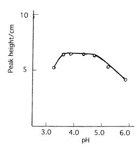
Fig. 2. Effect of sample solution pH on the peak height which is directly related to the adsorption efficiency for  $1.0 \text{ ng ml}^{-1}$  vanadium.
