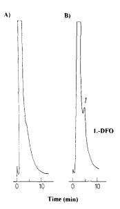
Fig. 4. Chromatograms of serum blank (A) and serum spiked with 50  $\mu$ g ml<sup>-1</sup> of DFO (B). Mobile phase contained 0.5% (w/v) Brij-35 in phosphate buffer 10<sup>-3</sup> M, pH = 7.4. Flow-rate, 1 ml min<sup>-1</sup>. Detection wavelength, 220 nm.
