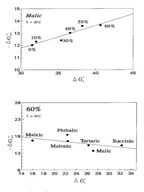
Fig. 3.  $\Delta G_{ass}^0 - \Delta G_2^0$  correlation for malic acid in different solvent compositions and  $\Delta G_{ass}^0 - \Delta G_1^0$  correlation in 60 wt% ethanol for different dicarboxylate ligands.
