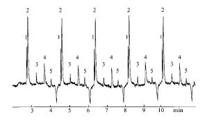
Fig. 5. Repeatability of the gas diffusion procedure, five consecutive injections (1.75 min interval). Conditions as in Fig. 3.
