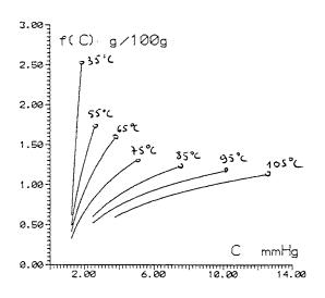
Fig. 3. Isotherms from 35 to 105°C silica gel (grain)—water L = 1 m,  $\Phi = 3/8$  inch,  $\omega = 2.5$  cc s<sup>-1</sup>, m = 0.250 ml.
