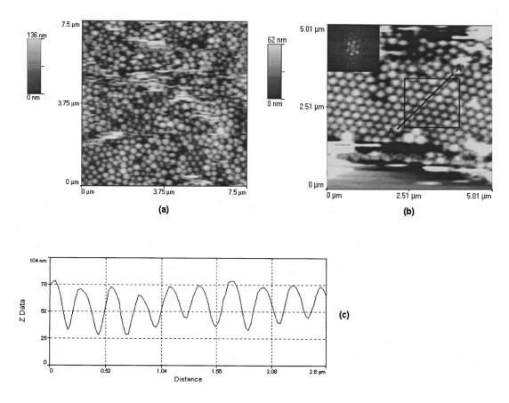
Fig. 1. AFM images of SM1 latex particles. (a) Disordered close packed regions; (b) hexagonal close packed region; (c) cross-sectional profile along AA' direction in (b). The AFM images were obtained in contact mode.
