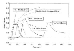
Fig. 5. Effect of reaction coil length and diameter on the signal from a biuret determination of bovine serum albumin. The dimensions given are the length and the diameter of the FIA reaction coil used in the assay.
