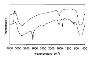
Fig. 1. FTIR spectra of SN5 (a) before and (b) after calcination.
