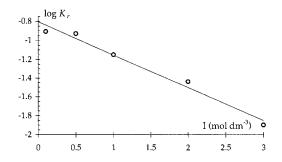
Fig. 7. Values of log  $K_r$  as a function of ionic strength. ( $\bigcirc$ ) experimental, ( $\longrightarrow$ ) theoretic using Eq. (17) and the values collected in Table 2.
