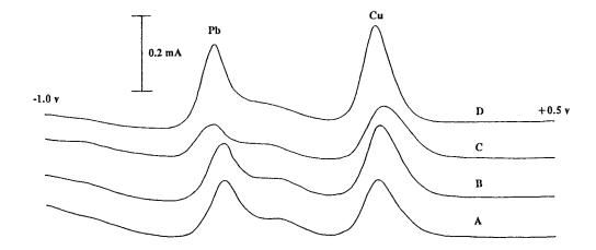
Fig. 2. Anodic stripping voltammograms of Pb(II) and Cu(II) measured by four peat moss electrodes incorporating different mesh-sized biomass. (A) 30-60 mesh; (B) 60-115 mesh; (C) 115-250 mesh; (D) > 250 mesh.
