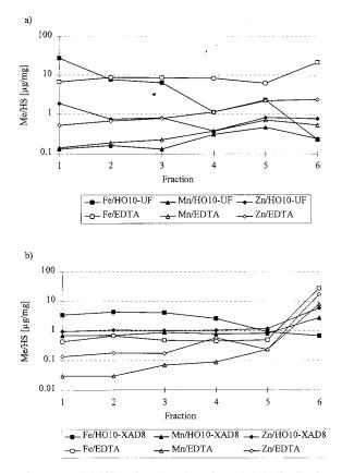
Fig. 4. EDTA lability of HS/metal species and their distribution in molecular size fractions obtained by MS-UF: (a) natural metal loading (HO10-UF); (b) synthetic metal loading (HO10-XAD8 loaded with 1.0  $\mu$ g mg<sup>-1</sup> each of Fe(III), Mn(II) and Zn(II)).
