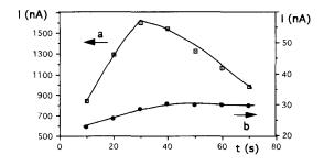
Fig. 4. Influence of the accumulation time on the AdS-SWV peak height for Nitralin solutions: (a)  $1 \times 10^{-8}$  mol  $1^{-1}$  and (b)  $4 \times 10^{-9}$  mol  $1^{-1}$ . For other conditions see Table 1.
