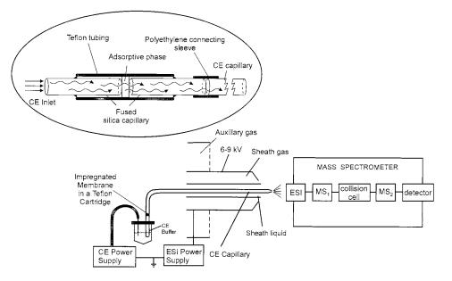
Fig. 1. Schematic of mPC-CE-MS using a Finnigan MAT ESI interface source. The mPC-CE cartridge is shown magnified for clarity (not to scale).
