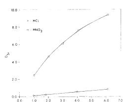
Fig. 5. Distribution ratio of  $Sr^{2+}$  as a function of aqueous acidity; [DCH18C6] = 0.1 M: diluent: 80% butanol-20% octanol, ( $\bigcirc$ ) HCl, ( $\Box$ ) HNO<sub>3</sub>.
