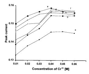
Fig. 3. The effect of the  $Cr^{3+}$  and  $Ca^{2+}$  concentration on the stripping peak: lead 0.05 µg ml<sup>-1</sup>; EDTA 10 mM ml<sup>-1</sup>. Calcium concentration: ( $\blacklozenge$ ) 0.0 M; ( $\blacksquare$ ) 0.02 M; (x) 0.04 M; ( $\bigtriangleup$ ) 0.06 M; ( $\blacksquare$ ) 0.08 M; (+) 0.10 M.
