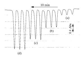
Fig. 8. Flow signals of silver(I).  $[Ag^{I}]$  (  $\times 10^{-7}$  mol dm<sup>-3</sup>) (a), 2.0; (b), 4.0; (c), 6.0; (d), 8.0. Conditions as in Fig. 1.
