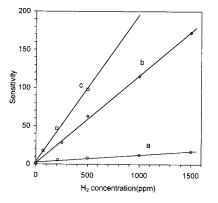
Fig. 7. Relationship between the sensitivity of (a) SN1, (b) SN6, and (c) SN5 sensors and  $H_2$  concentration at 573 K.
