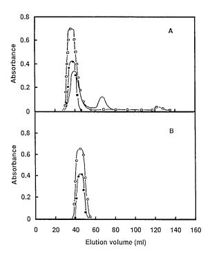
Fig. 1. (A) Elution pattern from a gel filtration column of the reaction product of glucose oxidase with activated PEG-Nleu. The eluate was analysed by reading at 280 nm ( $\bigcirc$ ) to detect the elution of the protein, by iodine reaction (—) to detect the PEG and by enzymatic activity ( $\bullet$ ). (B) Elution pattern of unmodified glucose oxidase. The eluate was analysed as in A.
