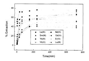
Fig. 4. Variation of % extraction of Ln(III) from a mixture containing eight lanthanide ions as a function of time at pH 5.5.  $[TTA]_0 = 3.2 \times 10^{-2}$  M,  $[K22DAP] = 8.0 \times 10^{-3}$  M,  $[La] = 2.70 \times 10^{-4}$  M,  $[Nd] = 3.04 \times 10^{-4}$  M,  $[Sm] = 3.01 \times 10^{-4}$  M,  $[Gd] = 2.63 \times 10^{-4}$  M,  $[Tb] = 3.03 \times 10^{-4}$  M,  $[Er] = 2.54 \times 10^{-4}$  M,  $[Yb] = 2.77 \times 10^{-4}$  M,  $[Lu] = 2.61 \times 10^{-4}$  M.
