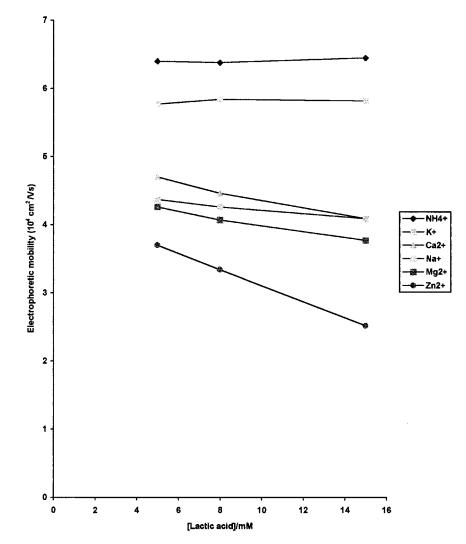
Fig. 4. The effect of combined use of lactic acid and 18-crown-6 ether on the differential electrophoretic mobility of the cations present in air particulate matters. [M] = 2 ppm,  $[NH_4^+] = 2$  ppm and BGE: 10 mM histidine and 2 mM 18-crown-6 (pH 4.65).
