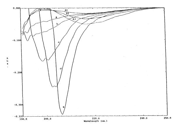
Fig. 1. First derivative UV-spectra for various concentrations of chitosan solutions. A1, 0.01 M acetic acid solution; A2, 0.02 M acetic acid solution; A3, 0.03 M acetic acid solution; a, 0.05 mg chitosan/0.01 M acetic acid solution; b, 0.10 mg chitosan/0.01 M acetic acid solution; c, 0.25 mg chitosan/0.01 M acetic acid solution; d, 0.50 mg chitosan/0.01 M acetic acid solution; e, 1.00 mg chitosan/0.01 M acetic acid solution.
