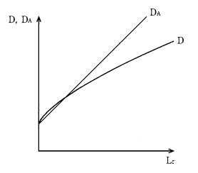
Fig. 10. Relationship among radial dispersion D, axial dispersion  $D_A$  and coil length  $L_r$ . Curve  $D_A$  versus  $L_r$  is calculated from  $\mu'_1 = 1.01$  in Eq. (3) (see text). Curve D versus  $L_r$  is the same as Fig. 4(b).
