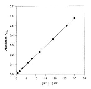
Fig. 3. Calibration graph for the determination or soluble GPO, using  $\alpha$ -GP as substrate.
