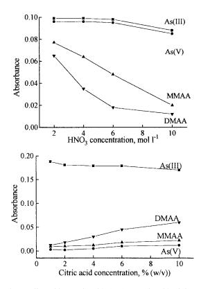
Fig. 2. Effect of inorganic acids (a-e), organic acids (f-j) and buffer systems (k-n) on the absorbance signals from 10 ng As of each arsenic species; other conditions as specified in Table 2.
