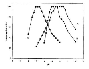
Fig. 1. Effect of pH on the extraction of trivalent gallium (A) (at  $5 \times 10^{-2}$  M sodium salicylate and 10 ml of 0.15% TPASO), indium (B) (at  $6.25 \times 10^{-2}$  M sodium salicylate and 5 ml of 0.5% TPASO) and thallium (C) (at  $6.25 \times 10^{-3}$  M sodium salicylate and 5 ml of 0.3% TPASO).
