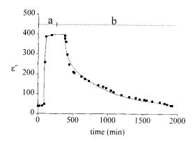
Fig. 7. Evolution of the dielectric losses  $\epsilon''$  of a 5.0 g silica gel column during the flow through of (a)  $5.9 \times 10^{-2}$  M NH<sub>3</sub> solution and (b) pure water, successively. Field frequency: 10 MHz.
