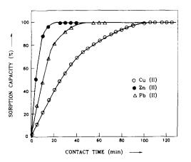
Fig. 4. Kinetics of Cu(II), Zn(II) and Pb(II) binding on Amberlite XAD-2-oVTSC. Cu(II): 10 ppm, 250 cm<sup>3</sup>, pH 3; Zn(II): 10 ppm, 250 cm<sup>3</sup>, pH 6; Pb(II): 10 ppm, 250 cm<sup>3</sup>, pH 6.5. Temperature:  $30^{\circ}$ C.
