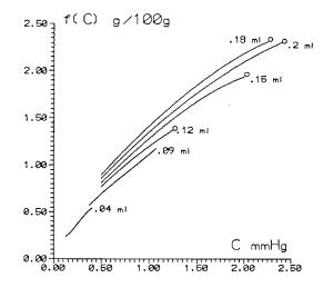
Fig. 8. Isotherms 100°C silica gel (grain)—methanol, L = 25 cm,  $\Phi = 3/8$  inch,  $\omega = 2.5$  cc s<sup>-1</sup>, m = 40, 90, 120, 150, 180 and 200 µl.
