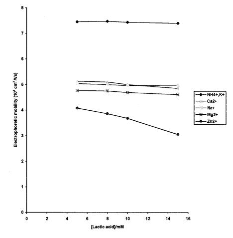
Fig. 3. The effect of using lactic acid alone on the differential electrophoretic mobility of the cations present in air particulate matters. [M] = 2 ppm,  $[NH_4^+] = 2$  ppm and BGE: 10 mM histidine (pH 4.65).
