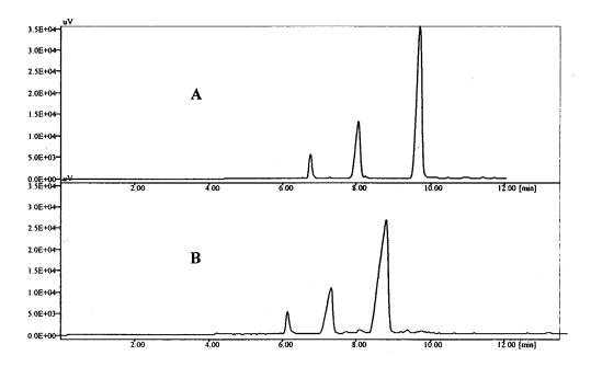
Fig. 4. Effect of pH on the separation of Pen G, 6-APA and phenyl acetic acid. (A) 40 mM borate (pH 9.4) as running buffer; (B) 40 mM borate  $+ H_3PO_4$  (pH 7.5) as running buffer. Other conditions of electrophoresis were the same as described in Fig. 3.
