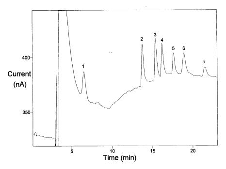
Fig. 6. Optimized determination of seven penicillins within a milk sample. NovaPak C-8 column. Waveform: given in Table 2B. Solvent program: given in Table 1C. All penicillins present prior to sample workup at  $1 \times 10^{-4}$  M: (1) ampicillin, (2) penicillin G, (3) penicillin V, (4) oxacillin, (5) cloxacillin, (7) dicloxacillin.
