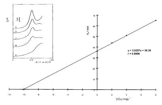
Fig. 4. Typical voltammograms and calibration curve of copper in a yeast wastewater sample. Curves: A, without ozone treatment; B, C, D ozone treatments for 30, 60 and 120 min, respectively; E as curve D after addition of 6  $\mu$ g l<sup>-1</sup> copper.
