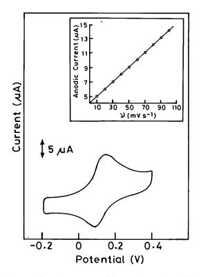
Fig. 1. Cyclic voltammogram of benzoquinone (Q) modified BPG electrode in phosphate buffer, pH 7.3. Scan speed:  $25 \text{ mV} \text{ s}^{-1}$ ; Plot of anodic peak current vs. scan rate for a Q modified BPG electrode in background electrolyte (inset).
