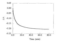
Fig. 3. Kinetic curve of the reaction between Ba-dimethylsulfonazo-III complex and sulphate ion in batch system; 2 ml of reagent solution plus 2 ml of sulphate ion solution  $(2 \text{ mg } 1^{-1})$ .
