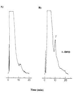
Fig. 3. Chromatograms of serum blank (A) and serum spiked with 60  $\mu$ g ml<sup>-1</sup> of DFO (B). Mobile phase contained 5% (v/v) Acetonitrile/0.1 M SDS in phosphate buffer 0.02 M, pH = 7.4. Flow-rate, 1 ml min<sup>-1</sup>. Detection wavelength, 210 nm.
