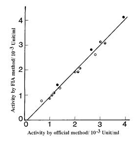
Fig. 5. Comparison between amylase activities obtained using the FIA method and the official method on various commerical digestive medicines.  $\bigcirc$ : A,  $\bullet$ : B,  $\Phi$ : C,  $\Phi$ : D,  $\Theta$ , E. The solid line is the regression line. The circles are the results of the digestive medicines.
