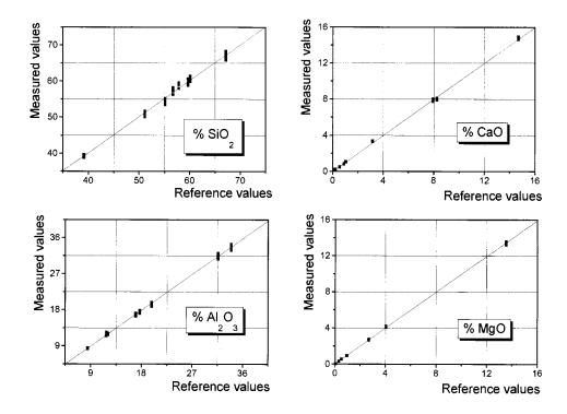
Fig. 4. Examples of plots of measured versus reference values for standard samples: the results of the different measures on the same solution are reported.
