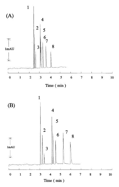
Fig. 5. The effect of PVA on the separation of a standard anion mixture. Conditions: (A) BGE: 5 mM Molybdate, 0.15 mM CTAH, 5 mM Tris buffer at pH 7.9; Capillary: 65 cm  $\times$  0.075 mm i.d. fused silica; Run: -20 kV; Current: 12  $\mu$ A; Injection: 8 cm for 20 s; Detection: 230 nm. (B) same as (A) except 0.01% PVA in BGE and Current: 10  $\mu$ A. Anion standards: 2 ppm each: 1 = chloride; 2 = sulphate; 3 = nitrate; 4 = fluoride; 5 = formate; 6 = phosphate; 7 = carbonate; 8 = acetate.
