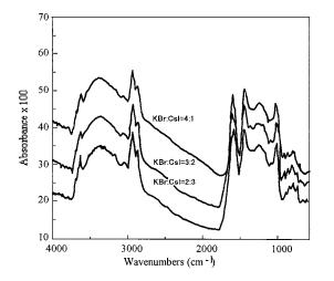
Fig. 10. Relation between KBr/CsI ratios and the background reduction effect of coal spectra.
