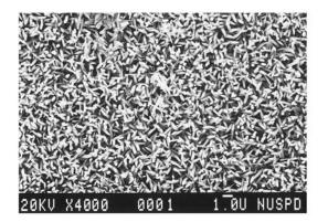
Fig. 1. SEM micrograph of ZnO thin film prepared by hydrothermal deposition showing a large number of the spikelike crystallites oriented normal to the substrate.
