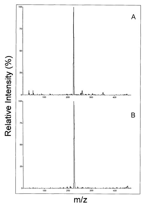
Fig. 9. Mass spectra from IMS/MS characterization of TNT at 1.6 ppm in a continuous stream of nitrogen without (A) and with (B) methylene chloride reagent gas.
