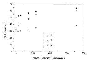
Fig. 2. Percentage extraction of Nd(III) and Lu(III) as a function of time at pH 5.5. A:  $[Nd] = 2.84 \times 10^{-4}$  M,  $[TTA]_0 = 8.0 \times 10^{-3}$  M,  $[K22DAP] = 1.0 \times 10^{-3}$  M; B:  $[Lu] = 2.66 \times 10^{-4}$  M,  $[TTA]_0 = 4.0 \times 10^{-3}$  M,  $[K22DAP] = 1.0 \times 10^{-3}$  M; C:  $[Nd] = 2.84 \times 10^{-4}$  M,  $[TTA]_0 = 4.0 \times 10^{-3}$  M,  $[K22DAP] = 1.0 \times 10^{-3}$  M,  $[K22DAP] = 1.0 \times 10^{-3}$  M.
