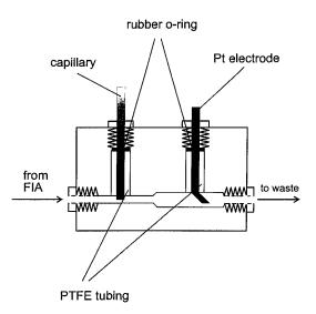
Fig. 1. Schematic view of the FIA-CE interface.
