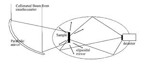
Fig. 15. Block diagram and profiles of light paths of a new accessory in FT-IR spectroscopy.
