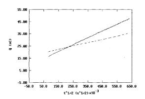
Fig. 4. Chronocoulometric dependence of charge on the square root of time for  $-4 \times 10^{-6}$  M TMpyP, potential step -0.1--0.8 V; - - 2 × 10<sup>-6</sup> M NiTMPyP, potential step: -0.8--1.2 V.
