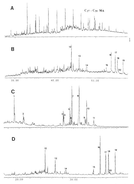
Fig. 2, BAL partial mass fragmentograms for: (A) m/z 253 (monoaromatic steroids: MA), (B) m/z 231 (triaromatic steroids: TA) from quadrupole GC-MS analysis; (C) m/z 253.1956 (MA); (D) m/z 231.1174 (TA) from high resolution GC-MS analysis.
