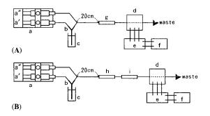
Fig. 1. Schematic diagram of microdialysis system without (A) and with amplification (B). (a) Two-channel microsyringe pump; (b) microdialysis probe; (c) sample solution; (d) amperometric detector [poly (1,2-diaminobenzene) film-coated platinum electrode]; (e) potentiostat; (f) recorder; (g) L-glutamate oxidase immobilized PTFE reactor; (h) saccharopine dehydrogenase immobilized PTFE reactor; (i) L-glutamate oxidase/glutamate dehydrogenase co-immobilized PTFE reactor.
