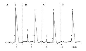
Fig. 6. Determination of acetic acid and sulphur dioxide in vinegar. Conditions: electrolyte II (chromate); 25 kV; acceptor solution: 5 mmol  $1^{-1}$  tris. Samples: A, common vinegar; B, apple cider vinegar; C, white wine vinegar; and D, red wine vinegar. Valve actuations at t = 0, 2.5, 5 and 7.5 min. Peaks: 1,  $SO_3^{2-}$ ; 2, acetate; \*, carbonate present in the acceptor phase.
