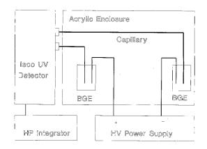
Fig. 1. Schematic diagram of the capillary electrophoresis system (HV power supply: Spellman 30 kV constant voltage supply; Detector: ISCO CE variable-wavelength detector; Recorder: HP3396A integrator; Capillary: 65 cm  $\times$  75  $\mu$ m i.d. uncoated fused-silica capillary).
