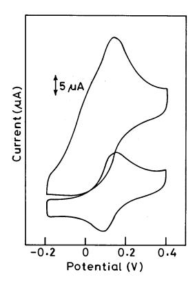
Fig. 2. (a) Cyclic voltammogram of Q modified BPG electrode in phosphate buffer, pH 7.3. (b) as in (a) with 8 mM NADH; Scan Rate:  $25 \text{ mV s}^{-1}$ .
