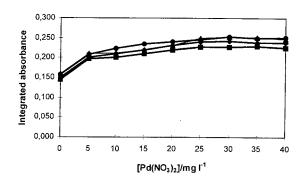
Fig. 2. Dependence of nickel absorbance signal with the amount of palladium nitrate for Ni<sup>2+</sup> aqueous standard ( $\blacklozenge$ ), synthetic sea water of high ( $\blacktriangle$ ) and low ( $\blacksquare$ ) salinity, and real sea water sample ( $\blacklozenge$ ).
