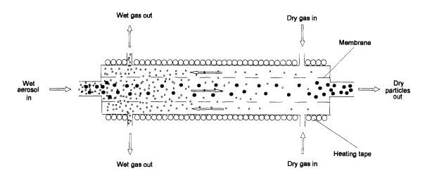
Fig. 3. The desolvation concept showing the fate of the analyte and solvent.
