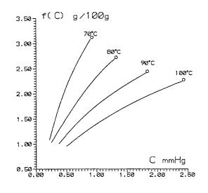
Fig. 7. Isotherms from 70 to 100°C silica gel (grain) methanol, L = 25 cm,  $\Phi = 3/8$  inch,  $\omega = 2.5$  cc s<sup>-1</sup>, m = 0.200 ml.
