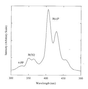
Fig. 5. Solid-matrix RTF spectra of 4-PP, B(f)Q, and B(a)P on Whatman 1PS paper after extraction of a water solution with 1PS filter paper.
