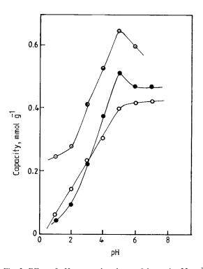
Fig. 2. Effect of pH on metal exchange. 0.1 g resin, 25 cm<sup>3</sup> reaction volume, equilibration time 24 h, copper, nickel and zinc concentration 200, 400, 400  $\mu$ g cm<sup>-3</sup> respectively. Copper,  $\bigcirc$  nickel,  $\bigcirc$  zinc.
