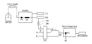
Fig. 1. On-line coupling of a subcritical water extractor with a FI manifold and an integrated retention-detection unit for the determination of iron in soils. PH, preheater; EC, leaching chamber; TC, temperature controller; RS, refrigerant system; VR, variable restrictor; DB, debubbler; R, reagent; E, eluent; PP, peristaltic pump; M, mixing point; L, mixing coil; SV, selecting valve; IV, injection valve; FC, flow-cell; W, waste.
