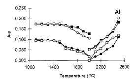
Fig. 2. Aluminium: Pyrolysis (left) and atomization (right) curves for hair slurries corresponding to the use of Pd ( $\Box$ ), Mg ( $\blacksquare$ ) and Pd-Mg ( $\bigcirc$ ) as chemical modifiers, and without chemical modification (•).
