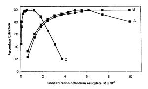
Fig. 2. Effect of sodium salicylate concentration on the extraction of trivalent gallium (A) (at pH 6.5 and 10 ml of 0.15% TPAS0), indium (B) (at pH 5.0 and 5 ml of 0.5% TPASO) and thallium (C) (at pH 3.0 and 5 ml of 0.3% TPAS0).
