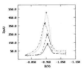
Fig. 2. Linear sweep voltammograms of  $1 \times 10^{-6}$  M NiTMpyP at different accumulation time  $t_A$ : (a) 2 s, (b) 10 s, (c) 60 s, (d) 90 s,  $E_A = -0.8$  V, scan rate 0.2 V s<sup>-1</sup>.
