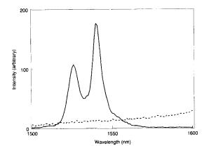
Fig. 4. Relative intensity of the light transmitted through six sheets of paper, measured with a 250 W halogen tungsten lamp based spectrophotometer (- - -), and with the EDFA based spectrophotometer (---).
