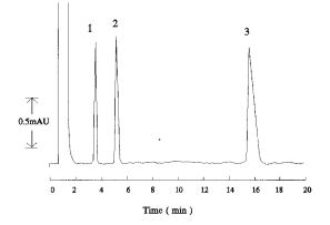
Fig. 11. The chromatogram of a typical rain water sample. Conditions: Eluent: 2 mM KHP at pH = 5.0; flowrate = 1.5 ml min<sup>-1</sup>; detection wavelength = 272 nm; sample volume = 0.100 ml; column = PRP-X100. Peaks: S = system peak; 1 = chloride; 2 = nitrate; 3 = sulphate.
