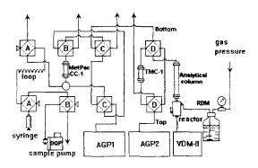
Fig. 1. Scheme of chelation ion chromatography system.
