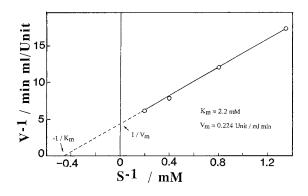
Fig. 3. Lineweaver–Burk plot for the hydrolysis reaction of starch by amylase. V, amylase activity; S, concentration of starch;  $K_{\rm m}$ , Michaelis constant obtained at the intercept of the extrapolated line with the abscissa;  $V_{\rm m}$ , maximum activity obtained at the intercept of the extrapolated line with the ordinate.
