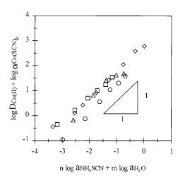
Fig. 5. Plot of log  $D_{\text{Co(II)}} + \log \alpha_{\text{Co(SCN)}_2}$  vs.  $n \log a_{NH_4SCN} + m \log a_{H_2O}$ , in the case of the extraction of Co(II) (initially  $10^{-3}$  M) by MIBK (98%) from NH<sub>4</sub>SCN ( $\diamondsuit$ ), NH<sub>4</sub>SCN/H<sub>2</sub>SO<sub>4</sub> 1 M ( $\square$ ), 1.5 M ( $\triangle$ ), 2 M ( $\bigcirc$ ) media. It is assumed that m = n = 3.
