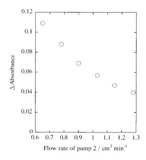
Fig. 6. Effect of flow rate of pump 2 on the FIA peak heights for silver(I).  $[Ag^{I}]$ ,  $5.0 \times 10^{-7}$  mol dm<sup>-3</sup>; extraction coil length, 3 m. Other conditions as in Fig. 1.
