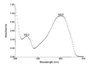
Fig. 2. UV absorption spectrum of chalcone in cyclohexane at  $25.0 \pm 0.1$  °C.
