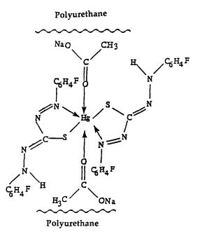
Fig. 1. A postulated structure of the mixed acetate  $F_2HDz$ -mercury(H) quasi complex on the polyurethane foam.
