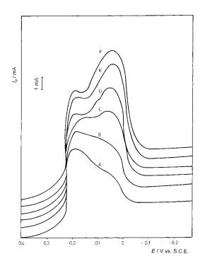
Fig. 2. Polarographic maxima of the oxygen reduction wave of a river water sample in dependence on the ozonolysis time. Curves A–F represent ozonolysis times of 0, 5, 10, 15, 30 and 60 min, respectively.
