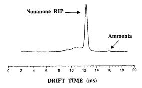
Fig. 1. Spectrum of ammonia in ethylene with 5-nonanone doping. To define the ammonia peak more clearly, 128 waveforms were averaged.
