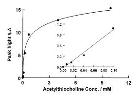
Fig. 5. Substrate response for RVC-agarose composite electrode. The electrode was based on RVC containing superporous agarose with immobilised acetylcholine esterase. The acetylthiocholine substrate (0.10 ml) at the concentration shown was injected and the response recorded.
