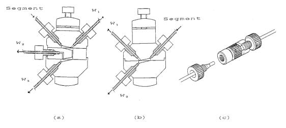
Fig. 2. Phase separators and connector of lines W1, W2, W3: exit of waste.
