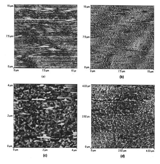
Fig. 3. AFM and LFM images of latex particles. (a) and (b) are AFM and LFM images of SM1 latex particles, respectively. (c) and (d) are AFM and LFM images of SM2 latex particles.
