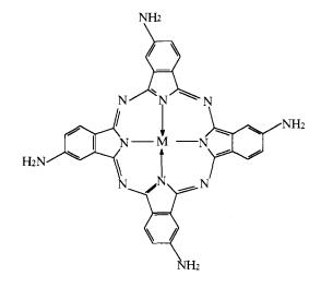
Fig. 1. Structure of M(II)-4,4',4",4'"-tetraaminophthalocyanine. M (II) = Nickel (II) or Copper (II).
