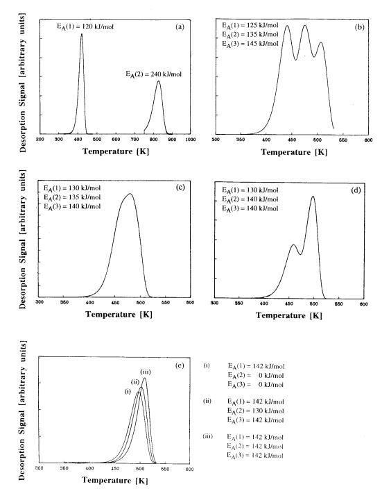
Fig. 5. Simulated TPDE curves for the successive loss of CO with different activation energies.
