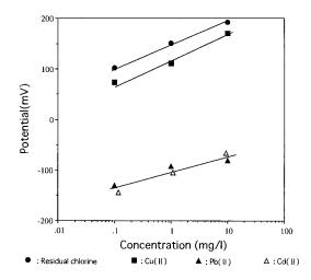
Fig. 4. Effect of heavy metal ions on the potential of the Pb(II)-ISE in the batch system.
