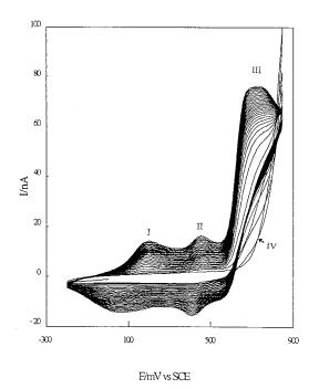
Fig. 1. The cyclic voltammograms at the microdisk gold electrode with 50 mV s<sup>-1</sup> in 0.5 M  $H_2SO_4$  containing 0.1 M aniline and  $5 \times 10^{-3}$  M 3,4-dihydroxybenzoic acid.
