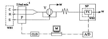
Fig. 1. Schematic flow diagram of the system. C, carrier; R, potassium periodate solution; S, sample; WB1, thermostatic water bath (30°C); WB2, sample compartment (15°C); P, peoristaltic pump; V, injection valve; FC, flow cell; W, waste; M, microcomputer; SP, spectrophotometer; CLB, the control circuit boad of the pump.
