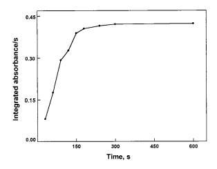
Fig. 6. Influence of the column loading time on the arsenic signal. Pre-concentration of 2.50  $\mu$ g 1<sup>-1</sup> As<sup>3+</sup> initial analytical solution in 0.1% (w/v) DDTP plus 5% (w/v) HCl.
