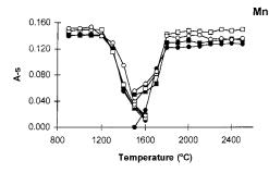
Fig. 3. Manganese: pyrolisis (left) and atomization (right) curves for hair slurries corresponding to the use of Pd ( $\Box$ ), Mg ( $\blacksquare$ ) and Pd-Mg ( $\bigcirc$ ) as chemical modifiers, and without chemical modification (•).
