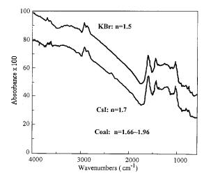
Fig. 3. Refractive indices of dilution materials and the profiles of transmission spectra of a coal.
