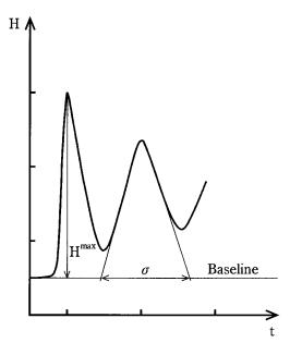
Fig. 2. Definition of signal height  $H^{\text{max}}$  and peak width  $\sigma$ .
