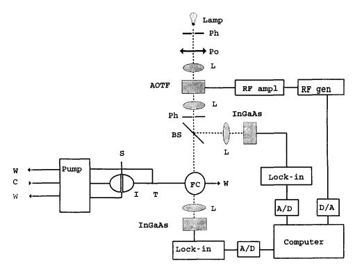
Fig. 8. Near-infra-red-FIA instrument: W, waste; C, carrier; Pump, peristaltic pump; S, sample; I, injector; T, T connector; FC, flow cell; Ph, pinhole; Po, polarizer; L, lens; BS, beamsplitter.
