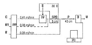
Fig. 1. Experimental set-up and FIA manifold. PP, peristaltic pump; W, waste; IV, injection valve; GPO, SBSR with immobilized GPO; D, detector; P, SBSR with plain beads; PC, personal computer; C, carrier (Tris–HCl 50 mmol  $1^{-1}$ ); S, sample ( $\alpha$ -GP or GPO in Tris–HCl 50 mmol  $1^{-1}$ ); R, reagent (AAP + DCPS + PO in Tris–HCl 50 mmol  $1^{-1}$ , pH 7.0); *R*1, reagent 1 ( $\alpha$ -GP 30 mmol  $1^{-1}$  in Tris–HCl 50 mmol  $1^{-1}$ , pH 7.8).
