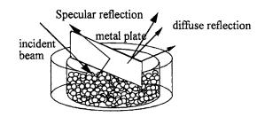
Fig. 4. Optics of diffuse reflection method (DRM).
