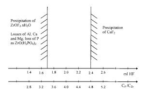
Fig. 3. Experimental results obtained by changing the amount of HF in the proposed dissolution procedure.
