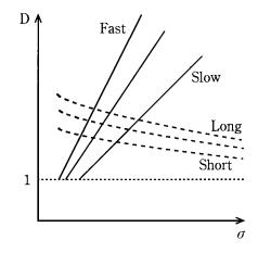
Fig. 9. Relationship between radial dispersion D and peak width  $\sigma$ . Solid line: Effect of flow-rate, Dotted line: Effect of coil length.
