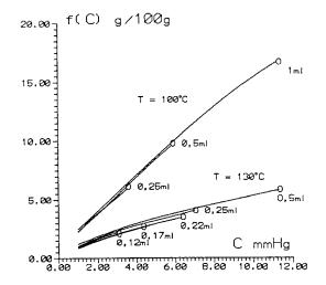
Fig. 9. Isotherms 100 and 130°C zeolite 4A (pellet)—water, L = 25 cm,  $\Phi = 3/8$  inch,  $\omega = 2.5$  cc s<sup>-1</sup>, T = 130°C, m = 120, 170, 220, 250, 500 µl, T = 100°C, m = 250, 500 and 1000 µl.
