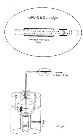
Fig. 2. A schematic diagram of the pressurized bomb apparatus used to load samples onto an mPC-cartridge prior to assembly of the mPC-CE capillary.
