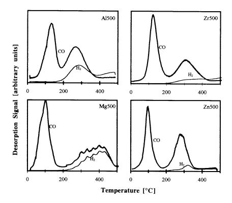
Fig. 3. TPDE of [Mo(CO)<sub>6</sub>] on ZnO, MgO, Al<sub>2</sub>O<sub>3</sub> and ZrO<sub>2</sub>; pretreatment 500°C; heating ramp 20°C min<sup>-1</sup>.
