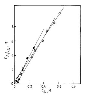
Fig. 6. Extended Langmuir adsoption isotherm.  $\bullet$  Copper,  $\bigcirc$  nickel,  $\odot$  zinc.
