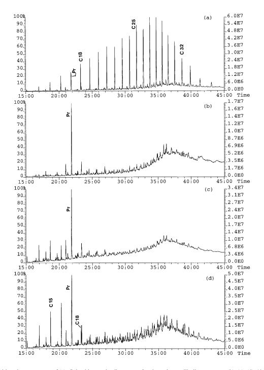
Fig. 4. Total ion chromatograms of (a): Columbian crude oil saturates fraction prior to silicalite treatment; (b), (c), (d): 10, 60 and 190 mg saturates fraction after silicalite treatment, analysed in full scan electron impact mode. x-axis: retention time in minutes; y-axis: peak intensity. (Pr = Pristane)
