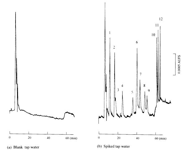
Fig. 3. Chromatogram of pesticides in spiked tap water sample: all the conditions and peaks are the same as shown in Fig. 2, concentrations of pesticides listed in Table 2.
