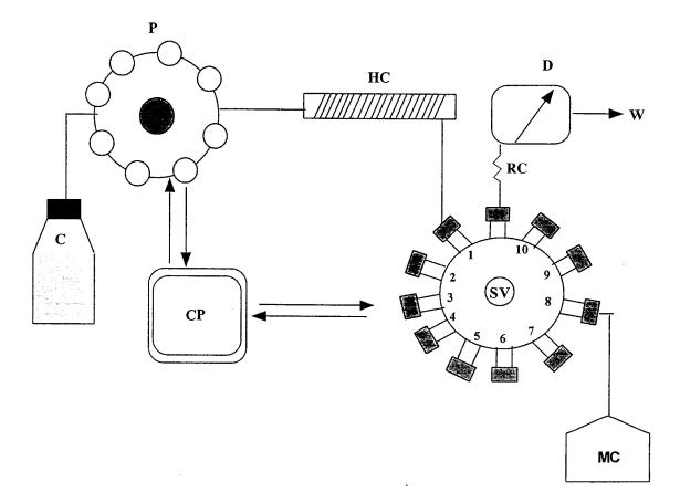
Fig. 1. SIA-manifold; C, carrier; P, peristaltic pump; HC, holding coil; SV, selector valve; RC, reaction coil; D, detector; CP, computer; MC, mixing chamber and W, waste.
