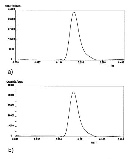
Fig. 4. Transient signal obtained by HG/FI - ICP/MS for a solution containing 1 µg  $1^{-1}$  of Se<sup>IV</sup> and 1 µg  $1^{-1}$  of total inorganic Se with: (a) before microwave treatment and (b) after microwave treatment.
