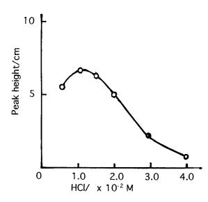
Fig. 4. Dependence of peak height for 1.0 ng ml<sup>-1</sup> vanadium adsorbed with 5 m sample loop on the concentration of HCl (as desorbing agent using 2.5 m loop).
