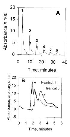
Fig. 7. SWE/WRP-LC of a 20 mg sample of unleaded gasoline on 2 ml of sand. All experimental conditions were the same as in Fig. 4 except that heartcuts were taken 5 min apart. (A) Depicts all six of the heartcuts taken while (B) illustrates the data for heartcuts one and six normalized to the same area and overlaid.
