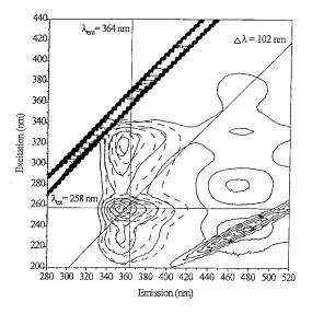
Fig. 2. Contours plots of the total fluorescence spectra of NA:  $\gamma$ -CD (----) and OH-NA:  $\gamma$ -CD (---) complexes. The selected paths for scanning the excitation ( $\lambda_{em} = 360$  nm), emission ( $\lambda_{ex} = 258$  nm) and synchronous ( $\Delta \lambda = 102$  nm) spectra are shown by the solid lines slicing the data matrix.
