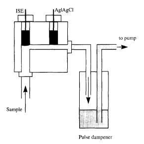
Fig. 1. Schematic diagram of the flow system, showing flow cell and pulse suppressor.
