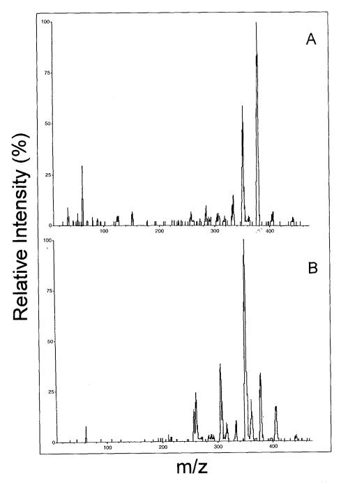
Fig. 11. Mass spectra from IMS/MS characterization of PETN at 1.1 ppm in a continuous flow of nitrogen without (A) and with (B) methylene chloride reagent gas.
