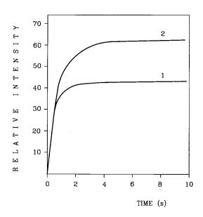
Fig. 2. Effect of the sample matrix on the kinetic curves obtained for the PABA system. Curve 1 was obtained from sample 2 (see Table 1), which was diluted up to a final 0.5  $\mu$ g ml<sup>-1</sup> PABA concentration; curve 2 corresponds to a standard solution containing 0.5  $\mu$ g ml<sup>-1</sup> PABA. [terbium(III)] = 2 × 10<sup>-3</sup> M; [TOPO] = 1.8 × 10<sup>-4</sup> M; [Triton X-100] = 0.1%; [hexamine buffer] = 2 × 10<sup>-2</sup> M.
