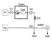
Fig. 1. Schematic of SWE/WRP-LC instrument. P1 and P2, water pump for SWE and WRP-LC systems, respectively; V1 and V2, needle valves; HC, heating coil; CC, cooling coil; Cell, SWE extraction cell; SV, switching valve; WRP, WRP-LC column; D, UV/VIS absorbance detector; AW, aqueous waste.
