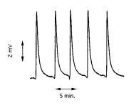
Fig. 7. FIA signals for residual chlorine obtained with the Pb(II)-ISE detector. Residual chlorine, 0.2 mg  $1^{-1}$ .
