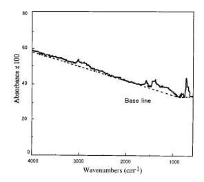
Fig. 1. Transmission spectrum of a coal tar pitch by KBr pellet method.
