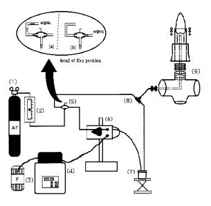
Fig. 1. Schematic diagram of the instrument assembly used. (1) Tank of argon; (2) carrier gas flow regulator; (3) fluoride ion solution; (4) peristaltic pump; (5) two-way key; (6) injection valve for fluoride solution; (7) reaction vessel; (8) three-port quick connector; (9) ICP torch.
