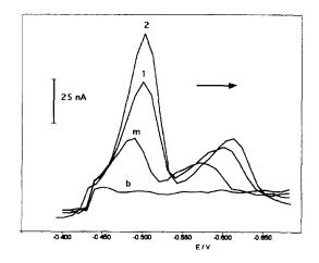
Fig. 5. AdS-DPV-voltammetric curves obtained after a cathodic scan, for the determination of Nitralin in ground-water. (b) blank, (m) ground-water spiked with Nitralin  $(4 \times 10^{-9} \text{ mol } 1^{-1})$ , (1) and (2) standard additions of 100 and 200 ml of  $1 \times 10^{-6} \text{ mol } 1^{-1}$  Nitralin solution. For working conditions see Table 1.
