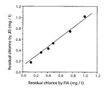
Fig. 8. Correlation between the JIS method and the FIA method for the determination of residual chlorine. Regression line, Y = 0.75X + 0.17; correlation factor, 0.967.
