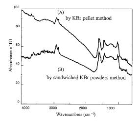
Fig. 7. The effect by sandwiched KBr powders to the spectral profile.
