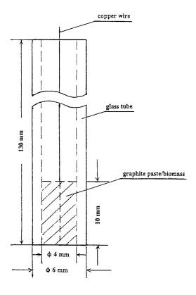
Fig. 1. Schematic of carbon paste/biomass electrode.
