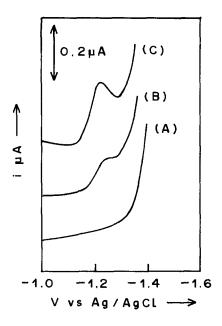
Fig. 2. Adsorptive stripping voltammetry of chromium in a gallium sample. Curve A: reagent blank; curve B: sample; curve C: sample plus standard addition, 10.4 ng ml<sup>-1</sup>. Media: 0.1 M TTHA, 0.05 M CH<sub>3</sub>COONa, 0.5 M NaNO<sub>3</sub>. Scan rate: 5 mV s<sup>-1</sup>; modulation amplitude: 50 mV; adsorption potential: -1.0 V (vs. Ag/AgCl); adsorption time: 30 s; rest time: 15 s.
