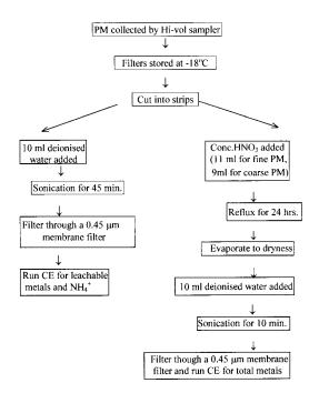
Fig. 7. Flowchart for sample preparation of air particulate matters (PM).
