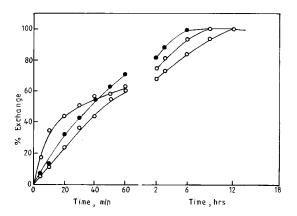
Fig. 4. Kinetics of metal exchange. 0.1 g resin, pH 5, 25 cm<sup>3</sup> reaction volume, equilibration time 24 h, copper, nickel and zinc concentration 200, 800, 400  $\mu$ g cm<sup>-3</sup> respectively. • Copper,  $\bigcirc$  nickel,  $\odot$  zinc.
