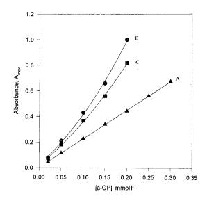
Fig. 4. Calibration graphs for  $\alpha$ -GP determination using GPO SBSR of different lengths: A = 5 cm, B = 10 cm and C = 20 cm.
