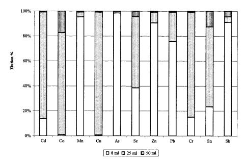
Fig. 2. Effect of eluent volume on the elution of sorbed elements (total amount of each element 400 µg).
