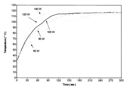
Fig. 3. Temperature curve in function of heating time in a focused microwave device (Working concentration 1  $\mu$ g 1<sup>-1</sup> Se<sup>VI</sup>; HCl concentration 6 mol 1<sup>-1</sup>).
