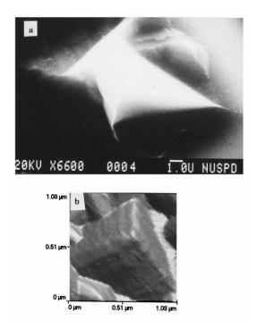
Fig. 4. Triangular conical tip images. (a) SEM micrograph of the noncontact tip showing irregular triangular conical shape; (b) AFM image of the tip apex obtained in noncontact mode.
