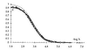
Fig. 4. Representation of Z vs.  $-\log h$ , for  $I = 1.0 \text{ mol dm}^{-3}$ in NaClO<sub>4</sub>. ( $\bigcirc$ ), ( $\diamondsuit$ )  $G_{tot} = 0.01 \text{ mol dm}^{-3}$ , ( $\square$ )  $G_{tot} = 0.005 \text{ mol dm}^{-3}$ , ( $\_$ ) theoretic considering the  $\beta$  and the  $K_r$  values, (- -) theoretic considering the  $\beta$  value.
