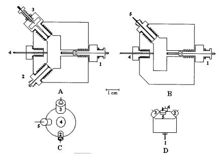
Fig. 1. Schematic of the wall-jet cell: A, B side elevation; C top view; D perspective view; 1, working electrode; 2, counter electrode; 3, reference electrode; 4, wall-jet nozzle; 5, liquid out.
