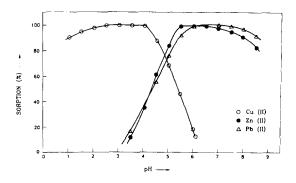
Fig. 2. Effect of pH on the sorption of Cu(II), Zn(II) and Pb(II). Cu(II): 1 ppm, 100 cm<sup>3</sup>, eluant 4 M HCl; Zn(II): 2 ppm, 100 cm<sup>3</sup>, eluant 2 M HCl; Pb(II): 2 ppm, 100 cm<sup>3</sup>, eluant 3 M HCl.
