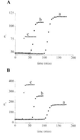
Fig. 6. Evolution of the dielectric permittivity  $\epsilon'$  (**A**) and the dielectric losses  $\epsilon''$  (**B**) of a 5.0 g silica gel column during the flow through of an aqueous ammonia solution. Breakthrough curves for three NH<sub>3</sub> concentrations:  $1.2 \times 10^{-2}$  M (**a**),  $5.9 \times 10^{-2}$  M (**b**) and  $2.3 \times 10^{-1}$  M (**c**). Flow rate: 1 ml min<sup>-1</sup>. Field frequency: 10 MHz.
