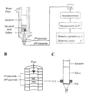
Fig. 1. Schematic representation of the experimental devices: A Capacitive axial cell and principle of dielectric measurements; **B** Transversal section of the cylindrical dielectric cell; **C** Chromatographic column with dielectric detector.
