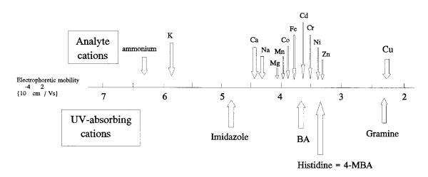
Fig. 5. The electrophoretic mobilities of common UV-absorbing cations and analyte cations.
