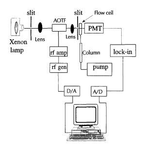
Fig. 6. Schematic diagram of the AOTF based detector for HPLC: PMT, photomultiplier tube; lock-in, lock-in amplifier; RF, RF power amplifier; RF gen, RF signal generator.
