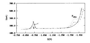
Fig. 7. Linear sweep voltammograms for: (a)  $3 \times 10^{-6}$  M NiTMpyP +  $5 \times 10^{-6}$  M DNA,  $t_A = 2$  s; (b)  $3 \times 10^{-6}$  M NiTMpyP +  $1.5 \times 10^{-5}$  M DNA,  $t_A = 2$  s; (c)  $3 \times 10^{-6}$  M NiTMpyP +  $1.5 \times 10^{-5}$  M DNA,  $t_A = 10$  s.
