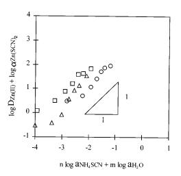
Fig. 6. Plot of  $\log D_{Zn(II)} + \log \alpha_{Zn(SCN)_2}$  vs.  $n \log a_{NH_4SCN} + m \log a_{H_2O}$ , in the case of the extraction of Zn(II) (initially  $10^{-3}$  M) by MIBK (98%) from NH<sub>4</sub>SCN ( $\bigcirc$ ), NH<sub>4</sub>SCN/H<sub>2</sub>SO<sub>4</sub> 1 M ( $\square$ ) and 2 M ( $\triangle$ ) media. It is assumed that m = 4 and n = 2.
