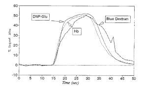
Fig. 8. Flow patterns by analyte molecular weight. The ByT-FAS system was used in a FIA operation mode. DNP-GLU is dinitropheny glutamic acid (mw = 341 Da), Hb is hemoglobin (mw = 66 kDa) and blue dextran ( $mw = \sim 1000$  kDa).
