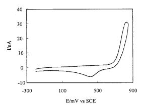
Fig. 2. The cyclic voltammograms at the microdisk gold electrode with 50 mV s<sup>-1</sup> in 0.5 M  $H_2SO_4$  containing  $5 \times 10^{-3}$  M 3,4-dihydroxybenzoic acid.
