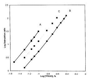
Fig. 4. Plots of log of distribution ratio vs. log of TPASO concentration for trivalent gallium (A) (at fixed pH 6.5 and  $5 \times 10^{-2}$  M sodium salicylate), indium (B) (at fixed pH 5.0 and  $6.25 \times 10^{-2}$  M sodium salicylate) and thallium (C) (at fixed pH 3.0 and  $6.25 \times 10^{-3}$  M sodium salicylate).
