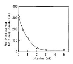
Fig. 4. Effect of L-lysine concentration in the carrier buffer on the enzymatic decomposition of 2-oxoglutarate in the saccharopine dehydrogenase immobilized reactor: sample,  $1 \times 10^{-5}$  M 2-oxoglutarate; carrier buffer, 0.1 M ammonium phosphate buffer (pH 7.2) held constant NADH concentration at 3 mM. The carrier buffer and Ringer's solution were pumped at same flow rate (2 µl min<sup>-1</sup>).
