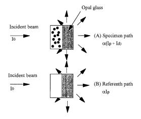
Fig. 5. Concept of opal glass method in visible region by Shibata.
