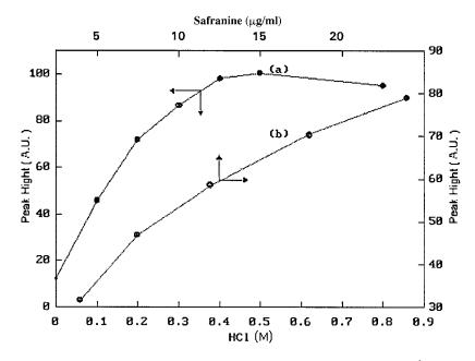
Fig. 3. Effect of safranine and HCl concentration on the peak height. Conditions: nitrite, 0.8  $\mu$ g ml<sup>-1</sup>; sample loop volume, 110  $\mu$ l; reaction coil length, 300 cm; flow-rate, 0.4 ml min<sup>-1</sup>;  $T = 25^{\circ}$ C; safranine 17  $\mu$ g ml<sup>-1</sup> (a); HCl 0.16 M (b).
