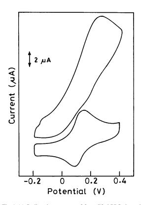
Fig. 4. (a) Cyclic voltammogram of Q modified BPG electrode in phosphate buffer, pH 7.3. (b) as in (a) with 5 mM  $AH_2$ ; Scan Rate: 25 mV s<sup>-1</sup>.
