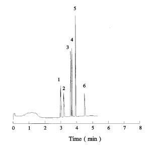
Fig. 6. The separation of a standard cation mixture. Conditions: BGE: 10 mM histidine, 2 mM 18-crown-6 and 8 mM lactic acid at pH 4.0; capillary: 65 cm  $\times$  0.05 mm i.d. fused silica; run: +20 kV; current: 9 uA; injection: 8 cm for 20 s; detection: 214 nm. Cation standards: 10 ppm each. 1, ammonium; 2, potassium; 3, calcium; 4, sodium; 5, magnesium; 6, zinc.
