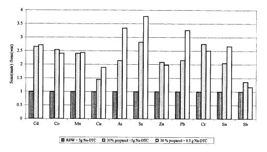
Fig. 4. Sensitivity of the ICP-AES analysis of propanol-water eluates containing dithiocarbamates of the studied elements.
