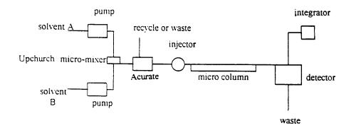
Fig. 1. Schematic of the capillary column HPLC system.
