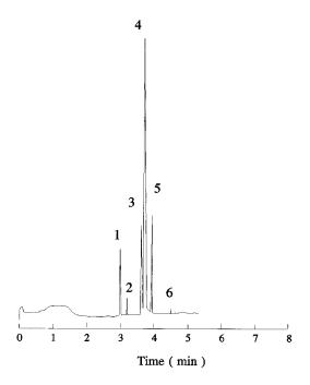
Fig. 8. A typical electropherogram showing the separation of leachable cations in a field sample of air particulate matters. Conditions: BGE: 10 mM histidine, 2 mM 18-crown-6 and 8 mM lactic acid at pH 4.0; capillary: 65 cm  $\times$  0.05 mm i.d. fused silica; run: +20 kV; current: 9 uA; injection: 8 cm for 20 s; detection: 214 nm. Migration order: 1, ammonium; 2, potassium; 3, calcium; 4, sodium; 5, magnesium; and 6, zinc.
