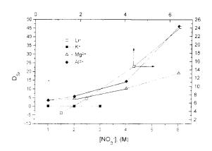
Fig. 6. Effect of inert metal nitrates on the distribution ratio of  $Sr^{2+}$ ; [DCH18C6] = 0.1 M; diluent: 80% butanol-20% octanol.
