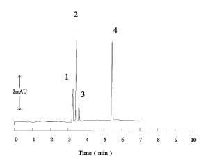
Fig. 14. The electropherogram of a typical rain water sample using hydrodynamic sampling for major anion determination. Conditions: BGE: 5 mM Molybdate, 0.15 mM CTAH, 5 mM Tris buffer at pH 7.9; Capillary: 65 cm  $\times$  0.075 mm i.d. fused silica; Run: -20 kV; Current: 10  $\mu$ A; Injection: 8 cm for 60 s; Detection: 230 nm. Migration order: 1 = chloride; 2 = sulphate; 3 = nitrate; 4 = carbonate.
