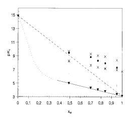
Fig. 4.  $pK_1$  versus mole fraction of water,  $x_{w}$ , in acetonitrile– water mixtures. +, furosemide; \*, chlorthiazide; **I**, trichlormethiazide; ×, amiloride; **V**, citric acid. The dashed straight lines correspond to the ideal variation of the  $pK_1$ values for the citric acid.
