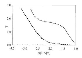
Fig. 7. Formation curves obtained for the Cu(II)/PAA  $3 \times 10^6$  system ( $\bigcirc$ ; R = 6.1) and for the Ni(II)/PAA  $3 \times 10^6$  system ( $\blacksquare$ ; R = 6.4) ( $C_A = 5.1 \text{ meq } 1^{-1}$ ).
