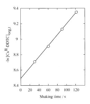
Fig. 4. A plot of  $-\ln[Cu^{II}-DDTC]_{org. t}$  against shaking time in the presence of  $2.0 \times 10^{-5}$  mol dm<sup>-3</sup> cobalt(II).
