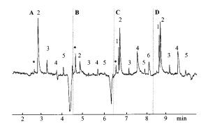
Fig. 4. Effect of different acceptor solutions: A, H<sub>2</sub>O; B, chromate (electrolyte I); C, 3 mmol  $1^{-1}$  borate; D, 5 mmol  $1^{-1}$  tris. Conditions were the same as in Fig. 3. Valve actuations at t = 0, 2, 4 and 6 min. Peaks: 1, HS<sup>-</sup>; 2, SO<sub>3</sub><sup>2-</sup>; 3, formate; 4, HCO<sub>3</sub><sup>-</sup>; 5, acetate; 6, borate.
