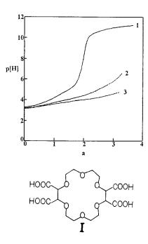
Fig. 1. Potentionetric equilibrium curves of TC18C6 (1), TC18C6.Al<sup>3+</sup> (2) and TC18C6.  $2Al^{3+}$  (3) at 25°C and ionic strength of 0.05 M. a = moles of base added per mole of ligand.
