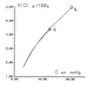
Fig. 11. Isotherms 100°C silica gel (powder)-water, L = 50 cm,  $\omega = 2.5$  cc s<sup>-1</sup>, m = 0.500 ml,  $\Phi = 3/8$  inch (1), 1/8 inch (2).
