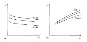
Fig. 5. Relationship between radial dispersion D and flow-rate  $Q_c$  at various coil length. (a) Result of ZCFIA, (b) Prediction by the present theory.
