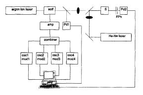
Fig. 2. Schematic diagram of the multiwavelength thermal lens spectrometer based on an AOTF as a polychromator: amp, RF power amplifier; osc, oscillator; mod, sinusoidal modulator; PIN, photodiode; F, interference filter; Ph, pinhole.
