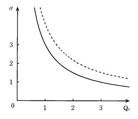
Fig. 12. Relationship between peak width  $\sigma$  and flow-rate  $Q_c$ . Solid line: Without the dispersion, Dotted line: With the dispersion.
