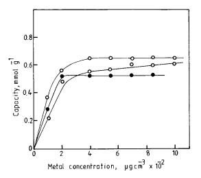
Fig. 3. Effect of metal ion concentration on % exchange. 0.1 g resin, pH 5, equilibration time 24 h, 25 cm<sup>3</sup> reaction volume. • Copper,  $\bigcirc$  nickel,  $\bigcirc$  zinc.
