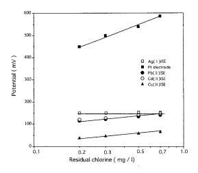
Fig. 3. Comparison of response to residual chlorine for the ISE and Pt electrode in the batch system.
