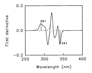
Fig. 3. Fist-derivative synchronous fluorescence spectra of pindolol (dotted line), propranolol (dashed line) and their mixture (solid line). Other conditions as in figure.
