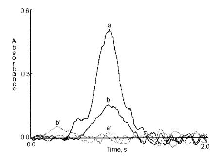
Fig. 2. Influence of palladium on the background and atomic pulses. after processing the solution in the flow system. Initial arsenic concentration: 2.00  $\mu$ g As 1<sup>-1</sup> (b) Without modifier (pyrolysis temperature of 200°C) and (a) with modifier (pyrolysis temperature of 1400°C); (---) Background signal, (—) atomic signal. Eluate collection in the 14–21 s interval and 120 s preconcentration time.
