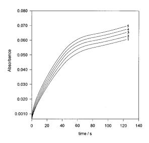
Fig. 3. Absorbance-time curves for the determination of the order of reaction with respect to ammonium ferric sulphate. [vitamin C] =  $5.6 \times 10^{-3}$  mol dm<sup>-3</sup>; [H<sub>2</sub>SO<sub>4</sub>] =  $1.79 \times 10^{-2}$  mol dm<sup>-3</sup>; [Fe<sup>3+</sup>] = (1)  $2.75 \times 10^{-4}$ ; (2)  $3.00 \times 10^{-4}$ ; (3)  $3.25 \times 10^{-4}$ ; (4)  $3.50 \times 10^{-4}$ ; (5)  $3.75 \times 10^{-4}$  mol dm<sup>-3</sup>; delay time,  $d_t = 12.0$  s.
