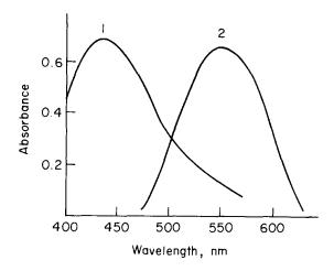
Fig. 1. Absorption spectra of BTDAB and its nickel complex (1) BTDAB against water. (2) Nickel complex against reagent blank.
