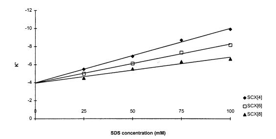
Fig. 3. Variation of capacity factor, k', of *p*-sulfonated calixarenes as function of SDS concentration.
