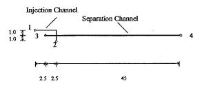
Fig. 1. Layout and dimensions of microfabricated channels. The separation channel is 50  $\mu$ m wide; the injection channel is 30  $\mu$ m wide; all the channels are 8  $\mu$ m deep; access holes are 1 mm in diameter. The dimensions shown are in mm.
