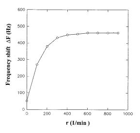
Fig. 1. Loading curve for QCM/Nafion (deposited from EtOH/H<sub>2</sub>O 80:20) in 0.5 mM Ru(bpy)<sub>3</sub><sup>+</sup> in 0.02 M phosphate buffer solution taken after 20 s, with increasing stirring speed.
