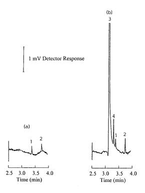
Fig. 1. Electropherograms of (a) standard anions by indirect detection. Peaks: 1 = nitrate; 2 = chlorate. (b) A real swimming pool water sample by indirect detection. Peaks: 1 = nitrate; 2 = chlorate; 3 = chloride; 4 = sulfate. Separation conditions: 10 mM chromate and 0.1 mM CTAB (pH = 9.4), -20 kV, 65 cm  $\times$  50 µm fused silica (52 cm to detector), 254 nm, 0.1 min injection time under 50 mbar, ambient temperature.
