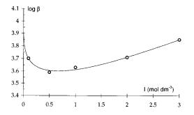
Fig. 6. Values of  $\log \beta$  as a function of the ionic strength. ( $\bigcirc$ ) experimental, ( $\longrightarrow$ ) theoretic using Eq. (16) and the values collected in Table 2.
