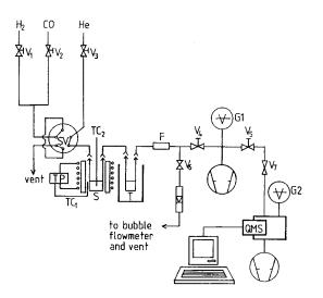
Fig. 1. Schematic diagram of the apparatus used for TPDE; F, 5  $\mu$ m filter; G<sub>1</sub>, G<sub>2</sub>, pressure gauges; QMS, quadrupole mass spectrometer; S, sample; SV, sampling valve; T, trap; TC<sub>1</sub>, TC<sub>2</sub>, thermocouples; TP, temperature programmer; V<sub>1</sub>–V<sub>6</sub>, fine-metering valves; and V<sub>7</sub>, metal-bellow valve (Nupro).
