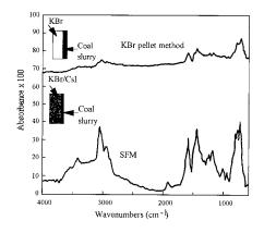
Fig. 17. IR spectra of a coal slurry (very viscous liquid) by KBr pellet method and SFM.
