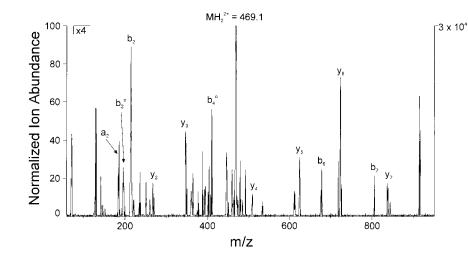
Fig. 4. mPC-tITP-CE-MS/MS analysis of an MHC class I peptide with a detected molecular ion of  $MH_2^{2+} = 469.1$ . All conditions as for Figure 3 except collision gas was xenon at a pressure of  $2 \times 10^{-5}$  mbar, ramped collision energy was 18-24 eV, scan range was 60-100 Da at 0.4 s/100 amu.
