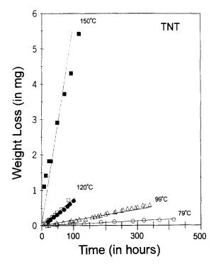
Fig. 2. Mass output for TNT at different temperatures. Each experiment including replicate experiments at a single temperature are given unique symbols:  $150^{\circ}C$  ( $\blacksquare$ ),  $120^{\circ}C$  ( $\bullet$ ,  $\Box$ ),  $99^{\circ}C$  ( $\triangle$ ),  $79^{\circ}C$  ( $\bigcirc$ ).
