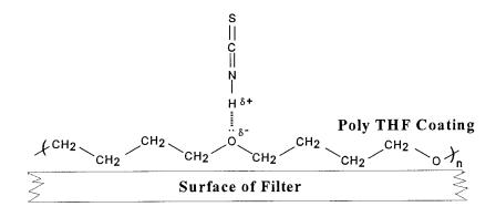
Fig. 5. Hydrogen bonding of thiocyanic acid (HSCN) to polyTHF.
