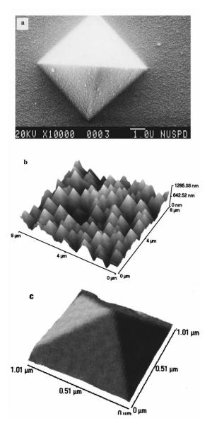
Fig. 2. Standard  $Si_3N_4$  tip images. (a) SEM micrograph of  $Si_3N_4$  tip. The dimensions of the tip are 5 µm in width and length; (b) AFM image of the tip consisting entirely of the tip pyramids. Note the sharp apex of the feature, which indicates the sharpness of both the tip and the crystallite apex; (c) single tip image obtained by zooming in on (b)
