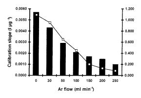
Fig. 1. Effect of different argon flow rates during the atomization step on the slope of aluminium calibration graph (bars) and aluminium absorbance from a hair slurry diluted 1:1 (line).
