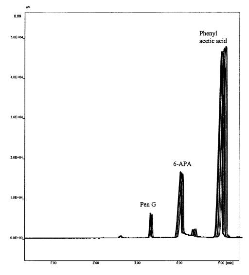
Fig. 7. Electropherograms of eight consecutive CE runs of one sample under the optimised conditions. CE conditions: capillary column, 43 cm total length/24 cm effective length/50  $\mu$ m I.D.; running buffer, 30 mM borate; voltage, 15 kV; column oven temperature, 30°C; injection, hydrodynamic/1 s at 12.7 cmHg pressure difference; UV detection, 210 nm.
