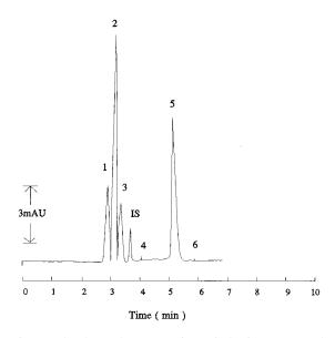
Fig. 13. The electropherogram of a typical rain water sample using electrokinetic sampling. Conditions: BGE: 5 mM Molybdate, 0.15 mM CTAH, 0.01% PVA and 5 mM Tris buffer at pH 7.9; Capillary: 65 cm  $\times$  0.075 mm i.d. fused silica; Run: -20 kV; Current: 10  $\mu$ A; Injection: -3 kV for 20 s. Migration order: 1 = chloride; 2 = sulphate; 3 = nitrate; 4 = fluoride; 5 = carbonate; 6 = acetate and IS = internal standard (chlorate, 500 ppb).
