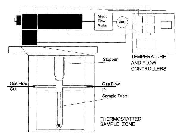
Fig. 1. Schematic representation of the Varian explosives vapor generator. Four zones are independently thermostatted and gas flow is delivered using a mass flow meter. Vapors are swept out of the generator through a heated outlet zone. All inner surfaces are glass.
