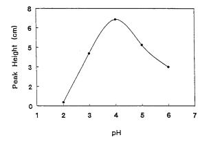
Fig. 5. Stripping peak heights of Pb(II) sorbed by a peat moss electrode at pH 2–6.
