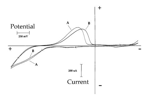
Fig. 2. Residual cyclic voltammograms of two different chromatographic solvents on gold. Solution deoxygenated with N<sub>2</sub>. Scan rate: 100 mV s<sup>-1</sup> (arrows denote scan direction). Rotation speed: 900 rpm. Traces: (A) 12% methanol/8% acetonitrile/80% 0.02 M acetate buffer (pH 4.7) (v/v); (B) 10% methanol/25% acetonitrile/65% 0.02 M acetate buffer (pH 4.7) (v/v).
