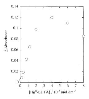
Fig. 5. Effect of Hg<sup>II</sup>-EDTA concentration on the FIA peak heights for silver(I). [Ag<sup>I</sup>],  $5.0 \times 10^{-7}$  mol dm<sup>-3</sup>; extraction coil length, 3 m. Other conditions as in Fig. 1.
