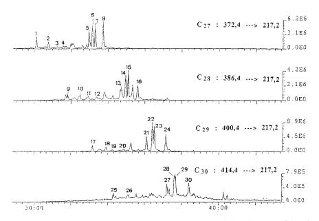
Fig. 3. BAL C27, C28, C29 and C30 steranes and diasteranes distribution obtained by MRM GC-MS-MS.
