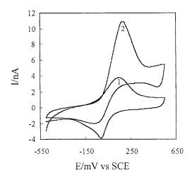
Fig. 4. The cyclic voltammograms at the composite polymer modified electrode in pH 7.0 buffer solution at a scan rate of 10 mV s<sup>-1</sup> in (a) absence and (b) presence of  $2.0 \times 10^{-3}$  M ascorbic acid.
