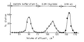
Fig. 7. Separation of copper, nickel and zinc.  $\bullet$  Copper,  $\bigcirc$  nickel,  $\odot$  zinc.
