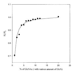
Fig. 2. Correction curve for GlcNac determination.
