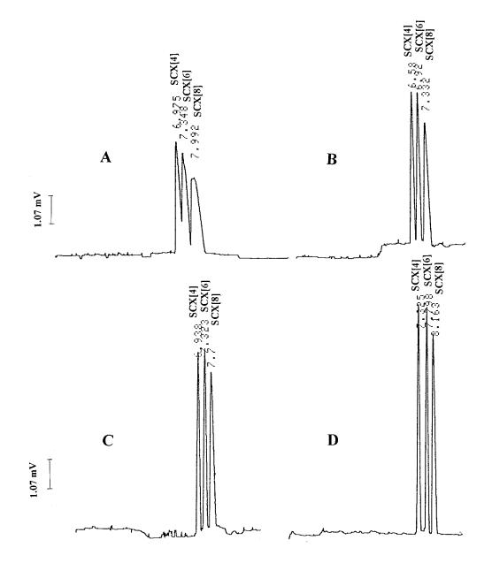
Fig. 1. Capillary electrophoresis separation of *p*-sulfonated calix[*n*]arenes, n = 4, 6, 8. Buffer: 25 mM boric acid/25 mM sodium borate, pH 9; separation capillary: 50 µm ID × 45 cm total length (effective length 30 cm); applied voltage: 18 kV; UV detection, 215 nm. Concentration of each peak is ~  $10^{-4}$  M. (A Without addition of SDS; (B) with addition of 25 mM SDS; (C) with addition of 50 mM SDS; (D) with addition of 75 mM SDS.
