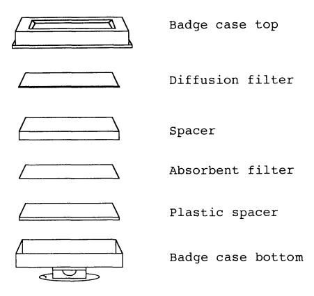
Fig. 2. Structure of a typical SO<sub>2</sub> passive sampler.
