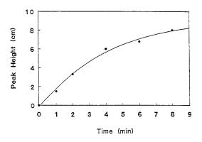
Fig. 6. Stripping peak heights of Pb(II) measured by a peat moss electrode after different deposition times.
