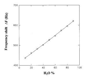
Fig. 3. Loading curves for QCM/Nafion in vigorous enough stirring solution of 0.5 mM Ru(bpy) $_3^{2+}$  in 0.02 M phosphate buffer solution taken after 20 s, as a function of the water percentage of the Nafion deposition solution.
