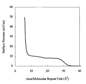
Fig. 1. Plot of surface pressure vs. area per molecule (adsorption isotherm) for mixed LB films consisting of PS-264 and stearic acid.
