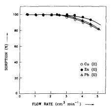
Fig. 3. Variation of percentage sorption with flow rate. Cu(II): 1 ppm, 100 cm<sup>3</sup>, pH 3; Zn(II): 2 ppm, 100 cm<sup>3</sup>, pH 6; Pb(II): 2 ppm, 100 cm<sup>3</sup>, pH 6.5.
