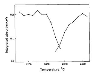
Fig. 3. Pyrolysis and atomization temperature curves after reduction and preconcentration. Initial arsenic concentration: 2.00  $\mu$ g l<sup>-1</sup>.
