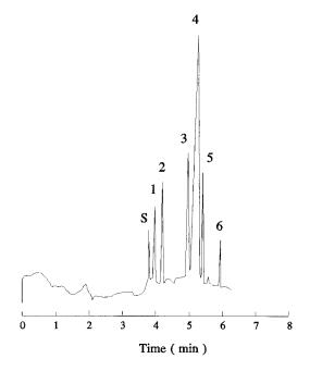
Fig. 9. A typical electropherogram showing the separation of cations in a field sample of air particulate matters after acid digestion. Conditions: BGE: 10 mM histidine, 2 mM 18-crown-6 and 8 mM lactic acid at pH 4.0; capillary: 65 cm  $\times$  0.075 mm i.d. fused silica; run: +15 kV; current: 8 uA; injection: 8 cm for 20 s; detection: 214 nm. Migration order: S, system peak; 1, ammonium; 2, potassium; 3, calcium; 4, sodium; 5, magnesium; and 6, zinc.
