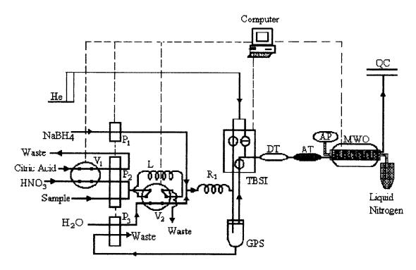
Fig. 1. Schematic diagram of the FI-Hg-AAS system used for the determination of arsenic species with on-line cryogenic trapping and volatilization with MW heating. The system is shown in the sample and nitric acid loading position for the determination of total inorganic arsenic, MMAA and DMAA.
