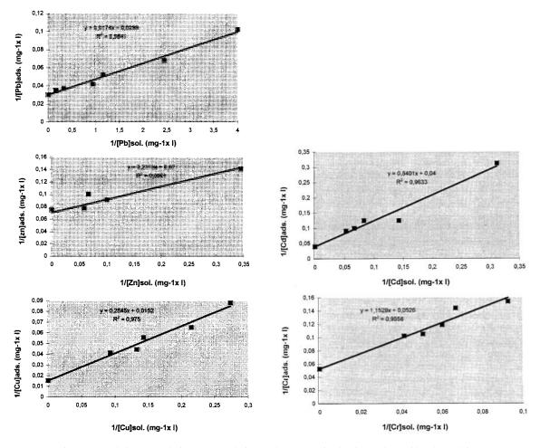
Fig. 2. (a) and (b) Interpolation curves relative to the Langmuir plot for each considered metal ion.
