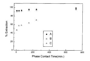
Fig. 3. Percentage extraction of Nd(III) and Lu(III) as a function of time at pH 8.0. A:  $[Nd] = 2.84 \times 10^{-4}$  M,  $[TTA]_0 = 8.0 \times 10^{-3}$  M,  $[K22DAP] = 1.0 \times 10^{-3}$  M; B:  $[Nd] = 2.84 \times 10^{-4}$  M,  $[TTA]_0 = 4.0 \times 10^{-3}$  M,  $[K22DAP] = 1.0 \times 10^{-3}$  M; C:  $[Lu] = 2.66 \times 10^{-4}$  M,  $[TTA]_0 = 4.0 \times 10^{-3}$  M,  $[K22DAP] = 1.0 \times 10^{-3}$  M.
