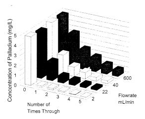
Fig. 6. The extraction of Pd(II) from solutions containing  $0.001 \text{ M NH}_4\text{SCN}/0.73 \text{ M HCl using different flow rates.}$
