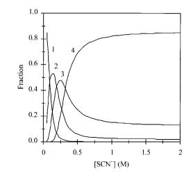
Fig. 4. Distribution plot of the species of the system  $Co(II)/SCN^{-}$ , calculated with the constants shown in Table 4. (1)  $Co^{2+}$ , (2)  $Co(SCN)^{+}$ , (3)  $Co(SCN)_2$ , (4)  $Co(SCN)_4^{2-}$ .
