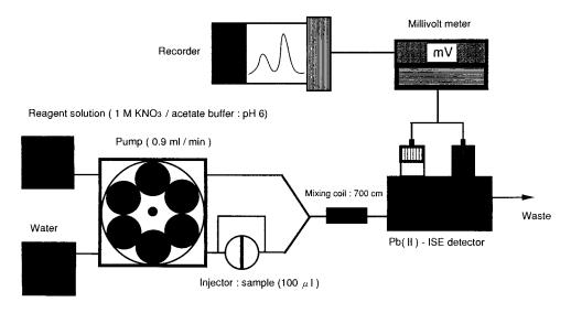
Fig. 2. Potentiometric flow injection system for residual chlorine.
