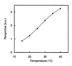
Fig. 5. Dependence of biosensor response on temperature in 1 mM glucose solution, pH 6.0.
