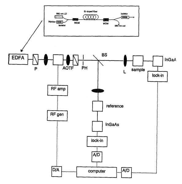
Fig. 3. Schematic diagram of the near infra-red spectrophotometer based on the use of the EDFA as a light source and AOTF as a dispersive element: EDFA, erbium doped fiber amplifier; P, polarizer; AOTF, acousto-optic tunable filter; PH, pinhole; BS, beamsplitter; L, lens; RF amp, RF power amplifier; RF gen, RF generator; InGaAs, detector. Insert: Schematic diagram of the erbium-doped fiber amplifier system: LD, laser diode; WDM, wavelength division multiplexer.
