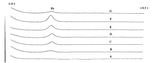
Fig. 9. Sorption-mode voltammograms of Pb(II) in a spiked water sample from Contraband Bayou measured by a peat moss electrode at different pH values. (A) blank; (B) pH 3.0; (C) pH 3.9; (D) pH 5.1; (E) pH 6.0; (F) pH 7.3; (G) pH 8.1.
