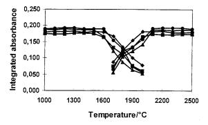
Fig. 1. Pyrolysis (left) and atomization (right) curves obtained for aqueous standard solution of 40  $\mu$ g l<sup>-1</sup> of Ni<sup>2+</sup> ( $\blacklozenge$ ), synthetic sea water samples of high ( $\blacktriangle$ ) and low ( $\blacksquare$ ) salinity ans real sea water sample ( $\blacklozenge$ ) spiked with Ni<sup>2+</sup> (40  $\mu$ g l<sup>-1</sup>).
