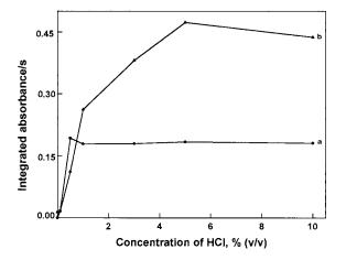
Fig. 4. Influence of HCl concentration on reduction and complexation of As(V). (a)  $1.00 \ \mu g \ l^{-1} \ As^{3+}$  analytical solution in  $0.1\% \ (w/v)$  DDTP without reducing agents; (b)  $2.50 \ \mu g \ l^{-1} \ As^{5+}$  analytical solution in  $0.1\% \ (w/v)$  DDTP plus  $0.5\% \ (w/v)$  KI and  $0.5\% \ (w/v)$  ascorbic acid. Reaction time: 30 min.
