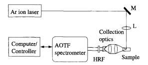
Fig. 1. Optical train for Raman spectroscopy with AOTF spectrometer.
