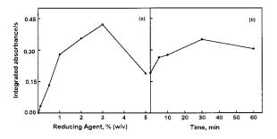
Fig. 5. Influence of KI-ascorbic acid addition (a) and reduction time (b) on As(V). The analytical solution was 2.00  $\mu$ g  $l^{-1}$  As<sup>5+</sup> in 0.1% (w/v) DDTP and 5% (v/v) HCl. The reduction time studies were carried out with 2.5% (w/v) KI and 2.5% (w/v) ascorbic acid.
