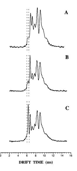
Fig. 2. Spectrum of ammonia in ethylene without a dopant. The vertical pairs of lines bracket the drift time of the ammonia peak. The other peaks are assumed to be clusters of ethylene and the reactant ion peak. (A) 0 ppm; (B) 0.1 ppm; (C) 1.5 ppm.
