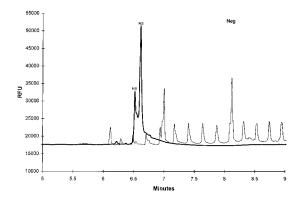
Fig. 4. The CE profile of an 'untreated' negative control sample. Two major non-specific (NS) 'contaminants' peaks are clearly evident. Run conditions were as in Fig. 2.
