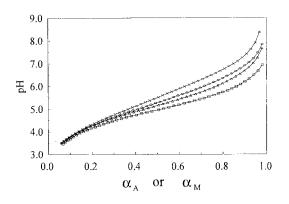
Fig. 4. Plot of pH versus the dissociation coefficient of PAA  $3 \times 10^6$  in the absence ( $\alpha_A$ , X) or in the presence ( $\alpha_M$ ) of Ni(II) for different values of *R* (*R* = 3.2  $\square$ ; 6.4  $\triangle$ ; 12.7  $\bigcirc$ ) (*C*<sub>A</sub> = 5.1 meq 1<sup>-1</sup>).
