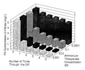
Fig. 3. The extraction of Pd(II) from solutions containing different NH<sub>4</sub>SCN concentrations and 0.73 M HCl. Experiment was performed on 100 ml of solution at 40 ml min<sup>-1</sup>.
