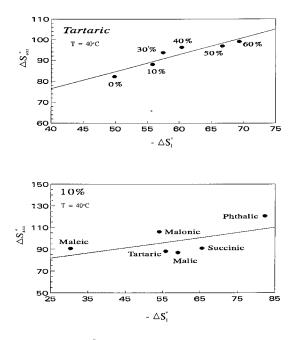
Fig. 1.  $\Delta S_{ass} - \Delta S_1^0$  correlation for tartaric acid in different solvent compositions and in 10 wt% ethanol for different dicarboxylate ligands.
