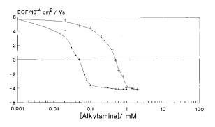
Fig. 2. The effect of alkylamine on EOF (BGE = 3 mM molybdate at pH 6.8).
