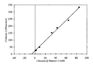
Fig. 4. Lineweaver–Burk plot of hexokinase velocity as a function of glucose concentration.  $K_{\rm m}$  of glucose with hexokinase calculated as the negative reciprocal of the *x*-intercept  $(-1/K_{\rm m})$ .
