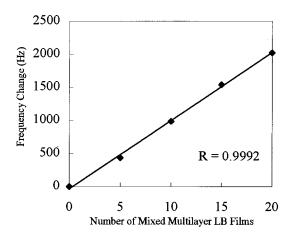
Fig. 2. Plot of frequency shifts vs. number of mixed multilayer LB films on the QCM.
