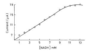
Fig. 3. Variation of catalytic current with concentration of NADH (Scan speed 25 mV s<sup>-1</sup>).
