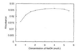
Fig. 4. Influence of sodium hydroxide in potassium bromide solution. Other reagents concentration: 0.1 M sodium hypochlorite; 15% potassium bromide; injection volume: 350  $\mu$ l.
