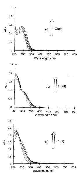
Fig. 1. The absorption spectral changes of (a) **3a**, (b) **3b** and (c) BPA  $(5 \times 10^{-5} \text{ mol dm}^{-3})$  in chloroform that was equilibrated with aqueous CuCl<sub>2</sub>  $(0-0.1 \text{ mol dm}^{-3})$ .
