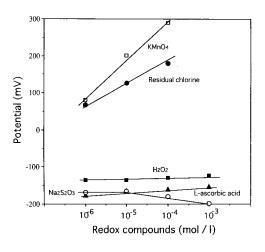
Fig. 5. Effect of redox compounds on the potential of the Pb(II)-ISE in the batch system.
