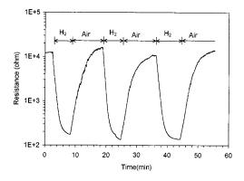
Fig. 5. Response transients of a SN5 sensor to switching on and off of 500 ppm  $H_2$  in air at 573 K.
