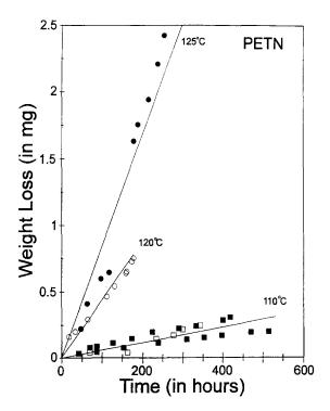
Fig. 4. Mass output for PETN at different temperatures:  $125^{\circ}C(\bullet)$ ,  $120^{\circ}C(\odot)$ ,  $110^{\circ}C(\Box, \boxtimes, \blacksquare)$ .
