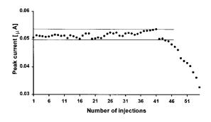
Fig. 6. Repeatability of a bare mercury film electrode for successive injections of whole blood samples in release agent  $(0.04 \text{ M Cr}^{3+}; 0.08 \text{ M Ca}^{2+})$
