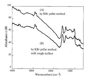
Fig. 6. The effect by using a rough surface KBr pellet to the spectral profile.
