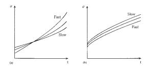
Fig. 7. Relationship between peak width  $\sigma$  and residence time *t* at various flow-rate. (a) Result of ZCFIA, (b) Prediction by the present theory.
