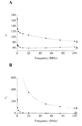
Fig. 3. Influence of the field frequency on the dielectric permittivity  $\epsilon'$  (**A**) and the dielectric losses  $\epsilon''$  (**B**) of 1.0 g silica gel in equilibrium with (**a**) 10 ml 0.46 M NH<sub>3</sub> and (**b**) 10 ml pure water.
