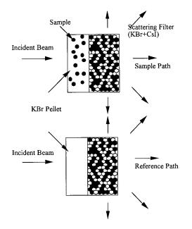
Fig. 9. Opal glass method with mixed alkalihalide pellet [scattering filter method (SFM)].
