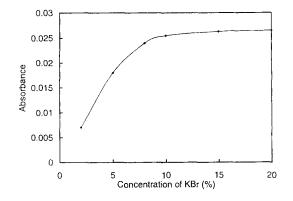
Fig. 3. Influence of concentration of potassium bromide. Other reagents concentration: 0.1 M sodium hypochlorite; the sodium hydroxide in potassium bromide solution is 4 M; injection volume:  $350 \mu l$ .
