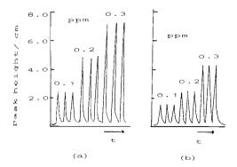
Fig. 7. Flow signals by different composition solvents. (a) (toluene + MIBK = 1 + 1); (b) (toluene + MIBK = 2 + 1).
