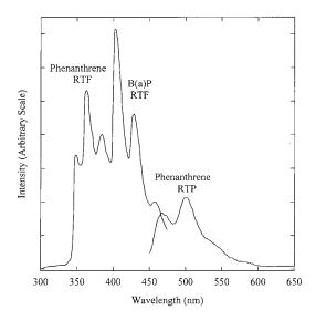
Fig. 4. Solid-matrix RTF spectra of B(a)P and solid-matrix RTF and RTP spectra of phenanthrene on Whatman 1PS filter paper after extraction of a water solution with 1PS filter paper.
