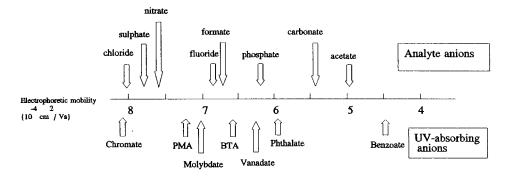
Fig. 3. The electrophoretic mobilities of common UV-absorbing anions and analyte anions.
