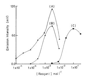
Fig. 2. Effect of reaction variables on pyridoxine catalysed reaction between luminol and  $H_2O_2$ . Variables: (A) luminol concentration; (B) hydrogen peroxide concentration; and (C) potassium hydroxide.
