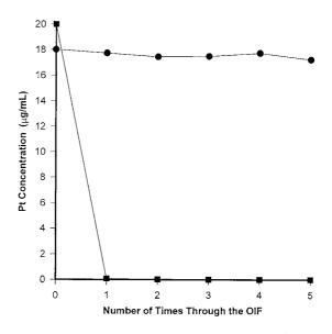
Fig. 8. The extraction of two solutions of 15 µg ml<sup>-1</sup> Pt(IV)/  $1 \times 10^{-3}$  M NH<sub>4</sub>SCN/ 0.73 M HCl at a flow rate of 100 ml min<sup>-1</sup>: •, Pt (IV) concentration present in the filtrate for a freshly prepared solution; ■, Pt (IV) concentration in the filtrate for a solution exposed to UV light to form the extractable complex.
