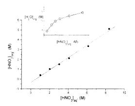
Fig. 2. Nitric acid concentration in the organic phase as a function of aqueous nitric acid concentration; diluent: 80% butanol-20% octanol. Inset: correlation between the organic phase water content and the concentration of nitric acid in the organic phase.
