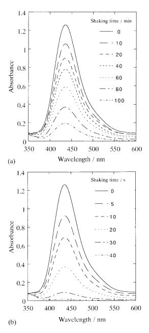
Fig. 2. Absorption spectra of the organic phase at various shaking times. (a), in the absence of free metal ion (pH = 6.9); (b), in the presence of  $3.9 \times 10^{-5}$  mol dm<sup>-3</sup> copper(II) (pH = 6.8).
