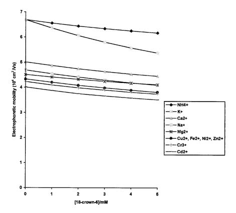
Fig. 2. The effect of using 18-crown-6 alone on the differential electrophoretic mobility of the cations present in air particulate matters. [M] = 2 ppm,  $[NH_4^+] = 2$  ppm and BGE: 10 mM histidine (pH 4.65).
