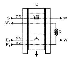
Fig. 1. Flow diagram of the system for arsenic determination. IC, injector-commutator; S, sample;  $E_1$ , water;  $E_2$ , ethanol; W, waste; L, ethanol sampling loop (150 µl); C-18, minicolumn; AS, autosampler cup; R, homogenization coil (25 cm, i.d. = 0.7 mm) Numbers in brackets equal flow rates in ml min<sup>-1</sup>. Arrows to the right show the directions of the solution flows. The arrow downwards indicates the movement of the central part of the injector-commutator.
