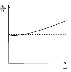
Fig. 11. Relationship between ratio of axial dispersion  $D_A$  to radial dispersion D and coil length  $L_r$ . Solid line: Result from computer-aided simulation (cf. [26] and [27]), Dotted line: Prediction of present theory.
