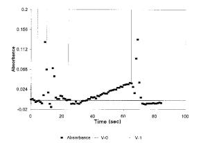
Fig. 9. The output of a ByT-FAS kinetic analysis of a bromocresol green assay of a  $0.1 \text{ mg ml}^{-1}$  of bovine serum albumin. Note the noise when the SIVs are fired. Three-way valve 0 was activated to divert the flow around the sample injection valve from 3 to 9 s and the three-way valve 1 was activated to divert the flow around the detector from 22 to 63 s.
