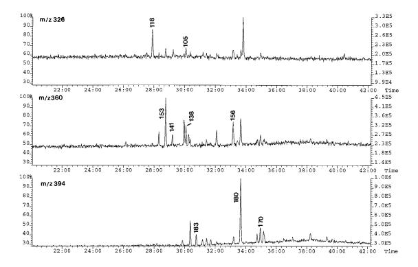
Fig. 3. NICI-GCMS mass chromatograms (m/z = 326, 360 and 394) of the Loch Ness sediment section after silicalite clean-up.  $\Sigma$ CB (22 congeners) = 1.4 ng g<sup>-1</sup> dry weight. Peak numbering identifies congeners. *x*-axis: retention time in minutes; *y*-axis: peak intensity.
