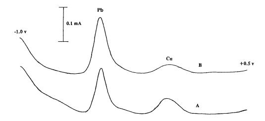
Fig. 3. Anodic stripping voltammograms of Pb(II) and Cu(II) measured by two Ramalina stenospora electrodes.
