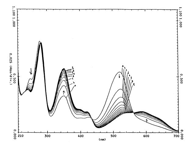
Fig. 2. Absorption spectra of safranine in the presence of 2  $\mu$ g ml<sup>-1</sup> of nitrite after (a) 30 s; (b) 100 s; (c) 170 s; (d) 240 s; (e) 310 s; (f) 380 s; (g) 450 s; and (h) 520 s from iniatiation of the reaction.
