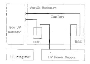
Fig. 1. Schematic diagram of the CE system (HV Power Supply: Spellman 30 kV constant voltage supply; Detector: ISCO CE variable-wavelength detector; Recorder: HP 3396A integrator; Capillary: 65 cm  $\times$  75 µm i.d. uncoated fused silica capillary).
