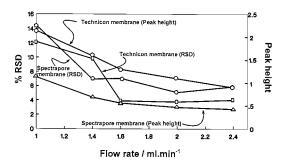
Fig. 4. Evaluation of response and relative S.D. as a function of the flow rate for both membranes.
