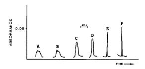
Fig. 3. Effect of various reagents on the precipitate dissolution: A, 0.5 M EDTA; B, 0.5 M sodium chloride; C, 1 M nitric acid; D, 1 M hydrochloric acid; E, 0.1 M ammonia; F, 0.5 M ammonium acetate. Washing solution: 30% ethanol.
