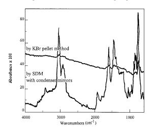
Fig. 14. Comparison of the spectra by KBr pellet method and SDM with condenser mirrors.
