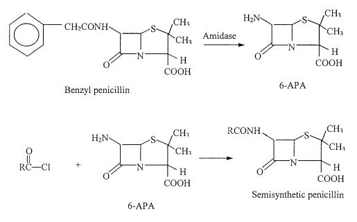
Fig. 2. Chemical reactions in manufacturing semisynthetic penicillins.
