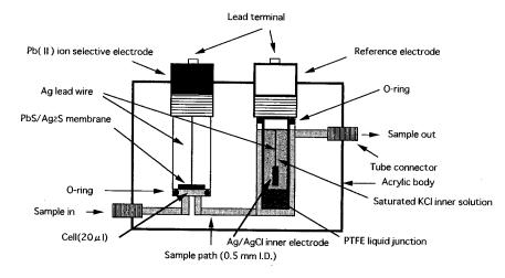
Fig. 1. Pb(II) ion-selective electrode detector for residual chlorine.
