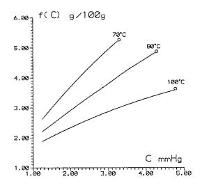
Fig. 6. Isotherms 70, 80 and 100°C silica gel (grain)—ethanol, L = 50 cm,  $\Phi = 3/8$  inch,  $\omega = 2.5$  cc s<sup>-1</sup>, m = 0.500 ml.
