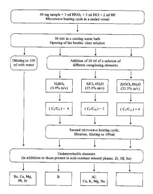
Fig. 1. Comparison of different methodologies of acid attack for the analysis of ceramic glazes.
