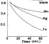
Fig. 3. Absorbance-time curves:  $2 \times 10^{-4}$ mol  $1^{-1}$  KIO<sub>4</sub>, 0.2 µg ml<sup>-1</sup>Mn(II), 0.2 µg ml<sup>-1</sup>Ag(I), 0.2 µg ml<sup>-1</sup>Fe(III), Other experimental conditions, as in Fig. 2.
