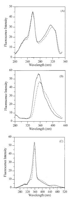
Fig. 3. A) Excitation ( $\lambda_{em} = 360$  nm), B) Emission ( $\lambda_{ex} = 258$  nm) and C) Synchronous ( $\Delta \lambda = 102$  nm) spectra data sets selected for the determination of NA and OH–NA, by PCR and PLS methods.
