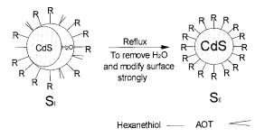
Fig. 2. Schematic illustration for the formation of strong surface modified CdS nanoparticles during reflux.
