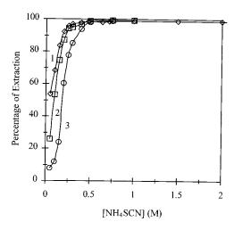
Fig. 3. Percentage of extraction of Zn(II) at equilibrium, at  $25 \pm 2^{\circ}$ C, as a function of NH<sub>4</sub>SCN concentration by MIBK (98%), in absence (1) and presence of H<sub>2</sub>SO<sub>4</sub> 1 M (2) and 2 M (3). Phase ratio = 1. [Zn(II)] was initially  $10^{-3}$  M.
