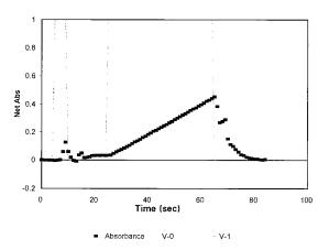
Fig. 7. A typical output of a ByT-FAS kinetic analysis. This is the output of a bromo-cresol green assay of 1.0 mg ml<sup>-1</sup> of bovine serum albumin. See Fig. 9 for the comparable output of the same assay of a 0.1 mg ml<sup>-1</sup> of bovine serum albumin. Three-way valve 0 was activated to divert the flow around the sample injection valve from 3 to 9 s and the three-way valve 1 was activated to divert the flow around the detector from 22 to 63 s.
