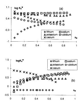
Fig. 3. Equilibrium quotient versus metal concentration in the resin phase for  $H^+ - M^+$  equilibria in Dowex CM-15 (a) and Dowex C650 (b).
