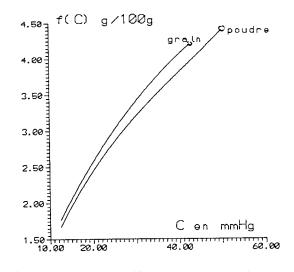
Fig. 12. Isotherms 100°C silica gel (powder (1), grain (2))-water, L = 50 cm,  $\Phi = 3/8$  inch,  $\omega = 2.5$  cc s<sup>-1</sup>, m = 0.500 ml.
