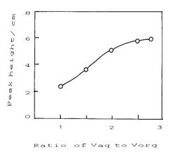
Fig. 8. Effect of the ratio of aqueous to organic phase volume SDS, 0.25 ppm; sample, 200  $\mu$ l; solvent, toluene + MIBK = 1 + 1.
