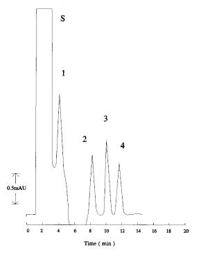
Fig. 12. The chromatogram for the determination of carbonate in a typical rain water sample. Conditions: Eluent: 0.6 mM KHP at pH = 9.5; flowrate = 1 ml min<sup>-1</sup>; detection wavelength = 272 nm; sample volume = 0.100 ml; column = PRP-X100. Peaks: S = system peak; 1 = chloride; 2 = nitrate; 3 = carbonate; 4 = sulphate.
