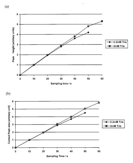
Fig. 7. The effect of sampling time on sensitivity for determining 5 ppm fluoride at different Tris buffer concentrations. (a = peak height, b = corrected peak area, Tris buffer concentration:  $\blacklozenge = 0.2 \text{ mM}$ ,  $\blacksquare = 5 \text{ mM}$ ).
