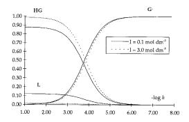
Fig. 5. Distribution diagram of D-gluconic- $\delta$ -lactone acid for I = 0.1 and 3.0 mol dm<sup>-3</sup> NaClO<sub>4</sub>.
