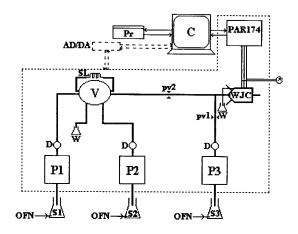
Fig. 2. Automated set-up for flow injection and detection by stripping voltammetry: C computer; D pulse dampeners; P1, P2, P3 pumps; PV1, PV2 pinch valves; S1, supporting electrolyte; S2, blood sample in release agent (1:15); S3, Hg<sup>2+</sup> plating solution; V Sampling valve with SL sample loop (100 μl); WJC wall-jet cell.
