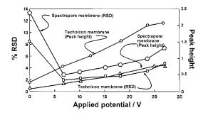
Fig. 3. Evaluation of response and relative S.D. as a function of the applied potential for both membranes.
