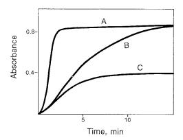
Fig. 2. Analytical signals obtained for (A) direct injection of 500 ng of Fe(III) in the FI system. (B) leaching of 500 ng of Fe(III) added to 0.13 g of diatomaceous earth under optimum working conditions. (C) leaching of 220 ng of Fe(III) from a soil.
