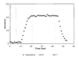
Fig. 6. A typical output of a ByT-FAS analysis of a reaction system that is in chemical equilibrium in the detector cell. Three-way valve 0 was activated to divert the flow around the sample injection valve from 0 to 6 s and the three-way valve 1 was activated to divert the flow around the detector from 21 to 42 s.
