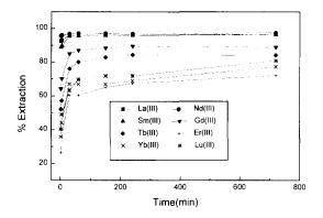
Fig. 5. Variation of % extraction of Ln(III) from a mixture containing eight lanthanide ions a function of time at pH 8.0.  $[TTA]_0 = 3.2 \times 10^{-2}$  M,  $[K22DAP] = 8.0 \times 10^{-3}$  M,  $[La] = 2.70 \times 10^{-4}$  M,  $[Nd] = 3.04 \times 10^{-4}$  M,  $[Sm] = 3.01 \times 10^{-4}$  M,  $[Gd] = 2.63 \times 10^{-4}$  M,  $[Tb] = 3.03 \times 10^{-4}$  M,  $[Er] = 2.54 \times 10^{-4}$  M,  $[Yb] = 2.77 \times 10^{-4}$  M,  $[Lu] = 2.61 \times 10^{-4}$  M.
