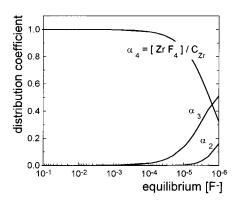
Fig. 2. Distribution diagram for zirconium (IV)-fluoride complexes.
