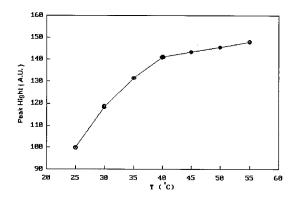
Fig. 5. Effect of temperature on the peak height. Conditions: nitrite,  $0.8 \ \mu g \ ml^{-1}$ ; sample loop volume, 110  $\mu$ l; reaction coil length, 300 cm; flow-rate, 0.4 ml min<sup>-1</sup>; safranine, 17  $\mu g \ ml^{-1}$ ; HCl, 0.5 M; KCl, 0.105 M.
