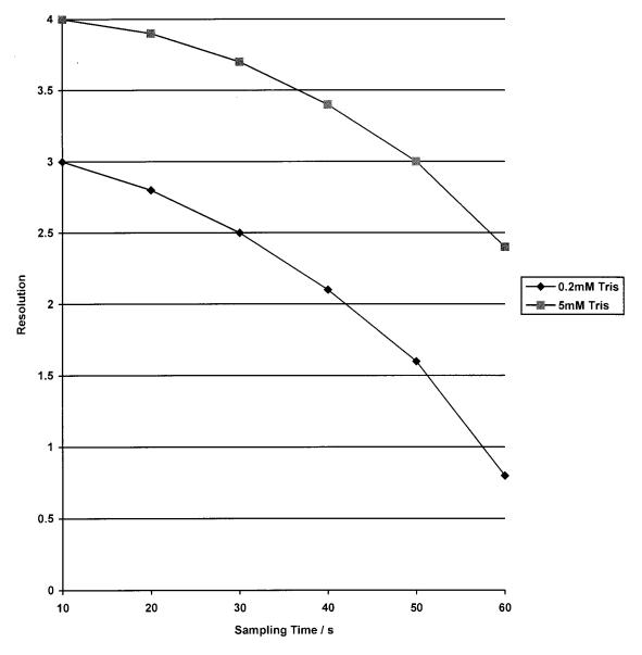
Fig. 6. The effect of sampling time on the resolution of 5 ppm of formate and fluoride at different Tris buffer concentration. Tris buffer concentration:  $\blacklozenge = 0.2 \text{ mM}$ ,  $\blacksquare = 5 \text{ mM}$ .
