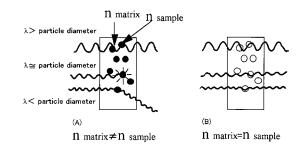
Fig. 2. Relationship between scattering and refractive indices (sample, matrix), scattering and wavelength or particle diameter.
