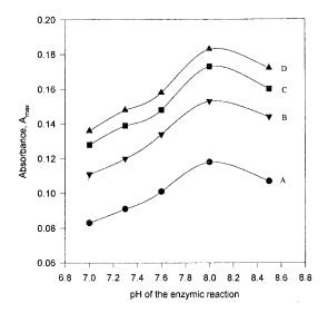
Fig. 2. Dependence of the efficiency of the enzymic system 'Immobilized GPO-soluble PO', from the pH, at varius concentrations of  $\alpha$ -GP:  $A = 0.010 \text{ mmol } 1^{-1}$ ,  $B = 0.020 \text{ mmol } 1^{-1}$ ,  $C = 0.030 \text{ mmol } 1^{-1}$  and  $D = 0.040 \text{ mmol } 1^{-1} \alpha$ -GP.
