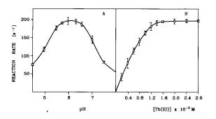
Fig. 1. Effect of pH (A) and terbium(III) concentration (B) on the system. [PABA] = 3  $\mu$ g ml<sup>-1</sup>; [terbium(III)] =  $1.5 \times 10^{-3}$  M; [TOPO] =  $10^{-4}$  M; [Triton X-100] = 0.1%. A  $2 \times 10^{-2}$  M hexamine buffer, pH 6, was used in (B).
