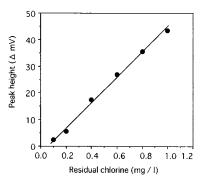
Fig. 6. Calibration curve for residual chlorine for the FIA system. Regression line, Y = 46.82X - 2.23; correlation factor, 0.996.
