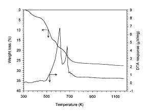
Fig. 2. TGA and DTA profiles of SN5 in flowing air with a heating rate of 20 K min<sup>-1</sup>.
