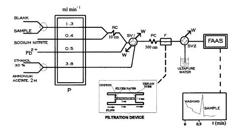
Fig. 1. Continuous precipitation-dissolution manifold for the indirect determination of sodium cyclamate. SV, switching valves; P, peristaltic pump; RC, reaction coil; PC, precipitation coil; W, waste lines; F, filter; FAAS, flame atomic absorption spectrometer.
