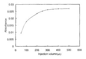
Fig. 5. Influence of injection volume. Reagents concentration: 0.1 M sodium hypochlorite; 15% potassium bromide is 4 M the sodium hydroxide solution.
