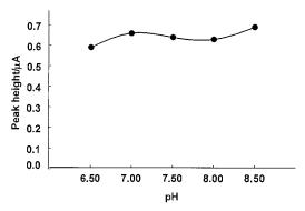
Fig. 2. Biosensor pH-optimum. The biosensor based on RVC coated with immobilised acetylcholine esterase was operated at different pH values by varying the transporting buffer (phosphate buffer with pH adjusted as indicated).
