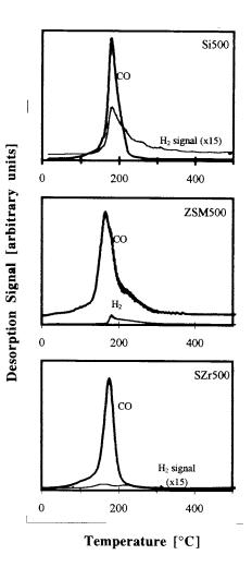
Fig. 2. TPDE of  $[Mo(CO)_6]$  on acidic supports; pretreatment 500°C; heating ramp 20°C min<sup>-1</sup>. Si, silica; ZSM, H-ZSM-5 molecular sieve; SZrO<sub>2</sub>, sulphated zirconia.
