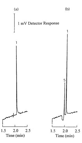
Fig. 2. Electropherograms of (a) standard anions by direct detection. Peak: 1 = nitrate. (b) A real sample by direct detection. Peaks: 1 = nitrate; 5 = not identified. Separation conditions: 10 mM sulfate and 0.1 mM CTAB (pH = 5.2), -20 kV, 65 cm × 50 mm fused silica (52 cm to detector), 214 nm, 0.1 min injection time under 50 mbar, ambient temperature.
