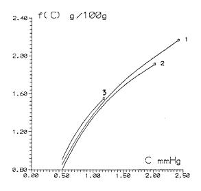
Fig. 10. Isotherms 100°C silica gel (grain)—methanol,  $\omega = 2.5$  cc s<sup>-1</sup>,  $\Phi = 3/8$  inch, m = 0.200 ml, L = 25 cm (1), 50 cm (2), 10 cm (3).
