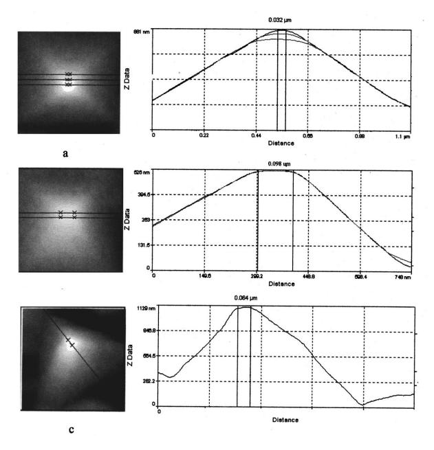
Fig. 5. Cross section profiles of the three different tips and measurements of the apex diameter of the tips. (a) standard  $Si_3N_4$ ; (b) broken supertip base; (c) triangular conical tip.
