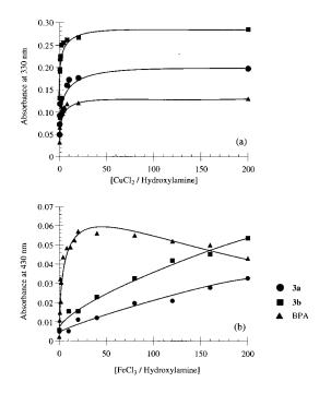
Fig. 3. The absorption spectral changes (Cu(II):  $\lambda = 330$  nm, Fe(III): 430 nm) of **3a**, **3b** and BPA induced by (a) Cu(II) and (b) Fe(III).
