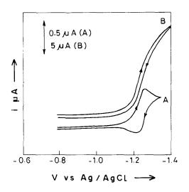
Fig. 1. Cyclic voltammograms of Cr(III)- TTHA. Curve A: 0.4 mM Cr(III), 0.02 M TTHA, 0.1 M CH<sub>3</sub>COONa, pH 6.2. Curve B: curve A plus 0.5 M NaNO<sub>3</sub>.
