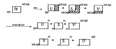
Fig. 5. SVD in the refinement of free concentration and binding parameters.
