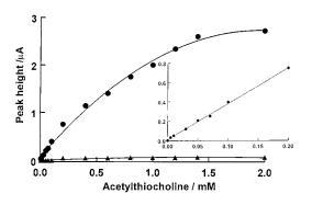
Fig. 3. Biosensor substrate response. The biosensor was based on RVC coated with immobilised acetylcholine esterase. The acetylthiocholine substrate (0.10 ml) at the concentration shown was injected and the response recorded.
