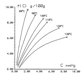
Fig. 5. Isotherms from 80 to 130°C zeolite 13X (pellet)—water, L = 25 cm,  $\omega = 2.5$  cc s<sup>-1</sup>,  $\Phi = 3/8$  inch, m = 0.350 m.
