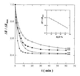
Fig. 4. Unloading curves for  $\text{Ru}(\text{bpy})_3^{2^+}$  from QCM/Nafion in a vigorously stirred 0.02 M phosphate buffer solution. The compositions of the deposition solutions are marked (as EtOH:H<sub>2</sub>O). Insert: loss of  $\text{Ru}(\text{bpy})_3^{2^+}$  after 1 min unloading, as a function of water content in the deposition solution.
