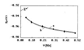
Fig. 6. Dependence of the peak potential  $E_p$  on the potential scan rate v for: (a)  $1 \times 10^{-6}$  M NiTMpyP pH 5.8; (b) a + 1 ×  $10^{-6}$  M DNA.
