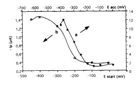
Fig. 3. Influence of the accumulation potential (a) and the start sweep potential (b) on the AdS-SWV peak height for a  $4 \times 10^{-6}$  mol  $1^{-1}$  Nitralin solution. For other conditions see Table 1.
