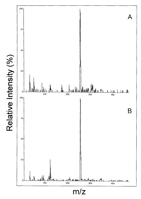
Fig. 10. Mass spectra from IMS/MS characterization of RDX at 1.5 ppm in a continuous flow of nitrogen without (A) and with (B) methylene chloride reagent gas.
