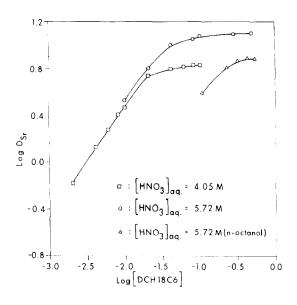
Fig. 4. Distribution ratio of  $Sr^{2+}$  as a function of DCH18C6 concentration in the mixed diluent  $(\Box, \bigcirc)$  and n-octanol  $(\triangle)$ .
