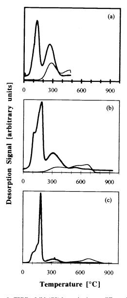
Fig. 8. TPDE of  $[Mo(CO)_6]$  on alumina at different Mo coverage; pretreatment temperature: 500°C, heating ramp: 20°C min<sup>-1</sup>, (a) 0.14 Mo nm<sup>-2</sup>; (b) 0.32 Mo nm<sup>-2</sup>; (c) 0.55 Mo nm<sup>-2</sup>.
