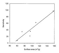
Fig. 6. Relationship between the surface areas of  $SnO_2$  sensors and their sensitivities to 500 ppm H<sub>2</sub> in air at 573 K.
