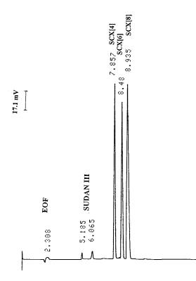
Fig. 2. Capillary electrophoresis separation of *p*-sulfonated calix[*n*]arenes, n = 4, 6, 8. Buffer: 25 mM boric acid/25 mM sodium borate/100 mM SDS pH 9; separation capillary: 50 µm ID × 50 cm total length (effective length 30 cm); applied voltage: -18 kV; UV detection, 215 nm. Concentration of each peak is  $\sim 10^{-4}$  M.
