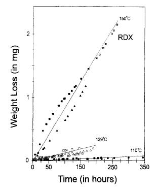
Fig. 3. Mass output for RDX at different temperatures: 150°C (shaded triangle, shaded square, shaded circle), 129°C ( $\triangle$ ,  $\Rightarrow$ ,  $\bigcirc$ ,  $\Box$ ), 110°C ( $\bullet$ ,  $\blacksquare$ ).
