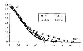
Fig. 2. Representation of Z vs.  $-\log h$ , at different waiting times for I = 0.5 mol dm<sup>-3</sup>. (-----) denotes the theoretical curve considering a monoprotic system with  $\log \beta \approx 3.6$ .
