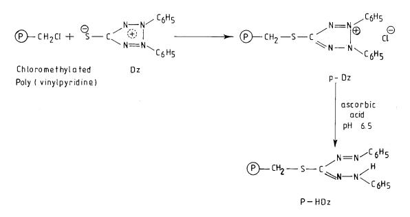
Fig. 1. Synthesis of the resin.  $D_z = dehydrodithizone$ ,  $HD_z = dithizone$ .
