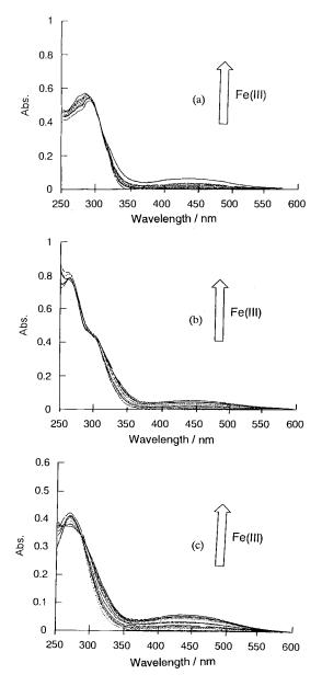
Fig. 2. The absorption spectral changes of (a) **3a**, (b) **3b** and (c) BPA  $(5 \times 10^{-5} \text{ mol dm}^{-3})$  in chloroform that was equilibrated with aqueous FeCl<sub>3</sub>  $(0-0.1 \text{ mol dm}^{-3})$ .
