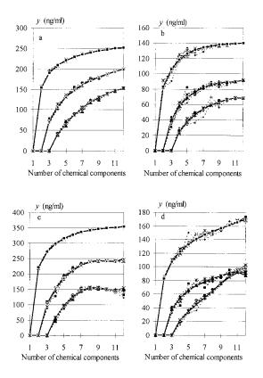
Fig. 8. Partial simulations. RMSE of PLS1 regression models using one to four latent variables. Dashed lines refer to the partial simulations with up to: 10, 25, 50, 75, 100, 125 and 150 mixtures. The full lines refer to the simulation with all possible mixtures. Noise-free simulations with five levels and 25 samples: (a) calibration and (b) validation. Simulations with added noise to absorbance data (0.05 AU) with two levels and 16 samples: (c) calibration and (d) validation.
