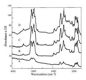
Fig. 13. Relation between spectral profiles and the sample powder size in SDM. A,  $<100 \mu$ m; B,  $<76 \mu$ m; C,  $<53 \mu$ m; D,  $<20 \mu$ m.
