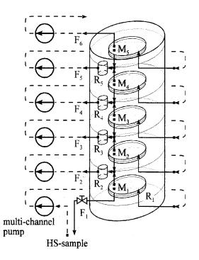
Fig. 2. Multistage ultrafiltration system (MS-UF) arranged as a filtration cascade.
