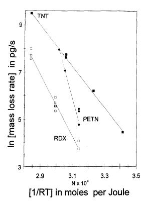
Fig. 5. Plots of ln(mass loss) versus 1/RT for TNT ( $\blacksquare$ ), RDX ( $\Box$ ), and PETN ( $\bullet$ ).
