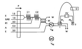
Fig. 2. Working principle of the gas diffusion-CE system. P, perstaltic pump; S, sample; R2, sodium hydroxide (optional solution); R1, sulphuric acid; A, acceptor solution; E, electrolyte solution; C1 and C2, reaction coils (60 cm, 0.5 mm i.d.); W, waste; M, gas diffusion membrane; Pt<sub>1</sub> and Pt<sub>2</sub>, platinum electrodes; HV, high voltage supply; D, detector; I, FIA-CE interface; B, buffer solution.  $V_{fill}$  shows injector in fill position,  $V_{ini}$  in inject position.
