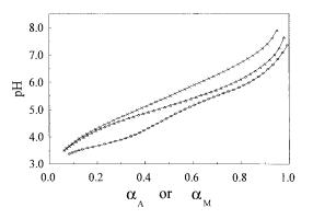
Fig. 1. Plot of pH versus the dissociation coefficient of PAA  $3 \times 10^6$  in the absence  $(\alpha_A; \mathbf{X})$  or in the presence  $(\alpha_M)$  of metal ion  $(\bigcirc, \text{Cu(II)}; \triangle, \text{Ni(II)}$  for very close values of  $R = C_A/C_M$   $(R = 6.1 \text{ and } 6.4, \text{ respectively; } C_A = 5.1 \text{ meq } 1^{-1}).$
