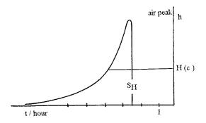
Fig. 1. Chromatogram of silica gel (powder)– water  $T = 60^{\circ}$ C, L = 50 cm,  $\Phi = 3/8$  inch,  $\omega = 2.5$  ccs<sup>-1</sup>, m = 0.5 ml.
