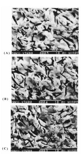
Fig. 5. Scanning electron microscope (SEM) micrographs of Nafion films formed from deposition solutions of various water contents. (A) 20%. (B) 40%. (C) 80%. The surface of the Nafion film was magnified 3600 times.
