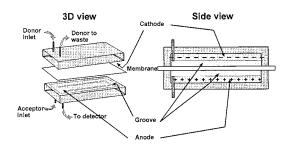
Fig. 2. A 3-D and side view of the electrodialyser unit.
