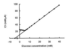
Fig. 6. Hanes plot of the calibration data for a glucose oxidase electrode.
